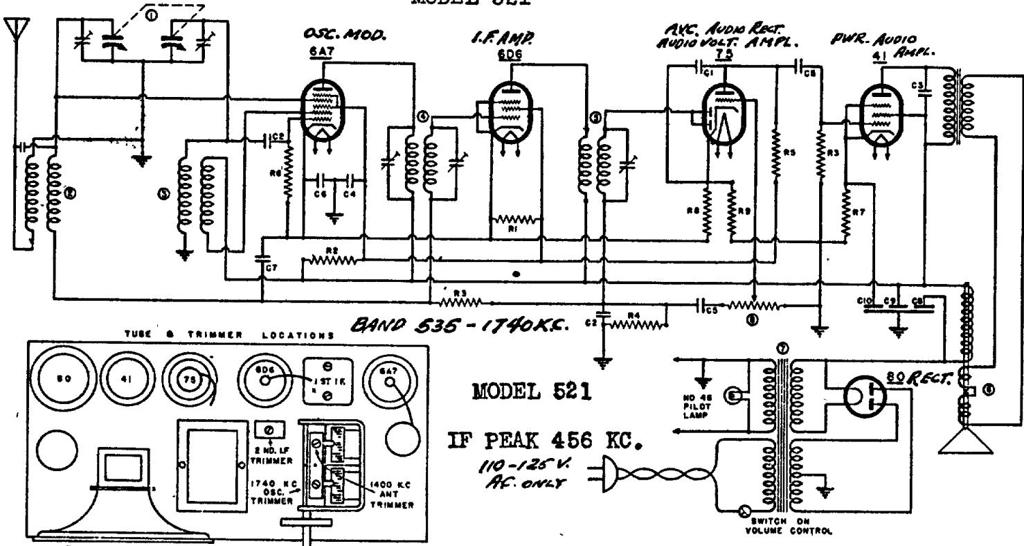
VOLTAGES MEASURED WITH 1000 OHM PER VOLT VOLTMETER.
