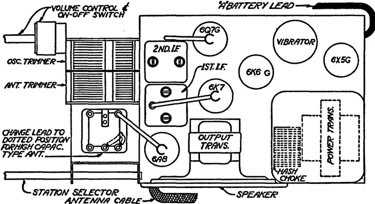
**GENERAL DATA.** The alignment of this receiver requires the use of a test oscillator that will cover the frequencies of 456, 600, 1400, 1550 and an output meter to be connected across the primary or secondary of the output transformers. If possible, all alignments should be made with the volume control on maximum and the test oscillator output as low as possible, to prevent the AVC from operating and giving false readings.
