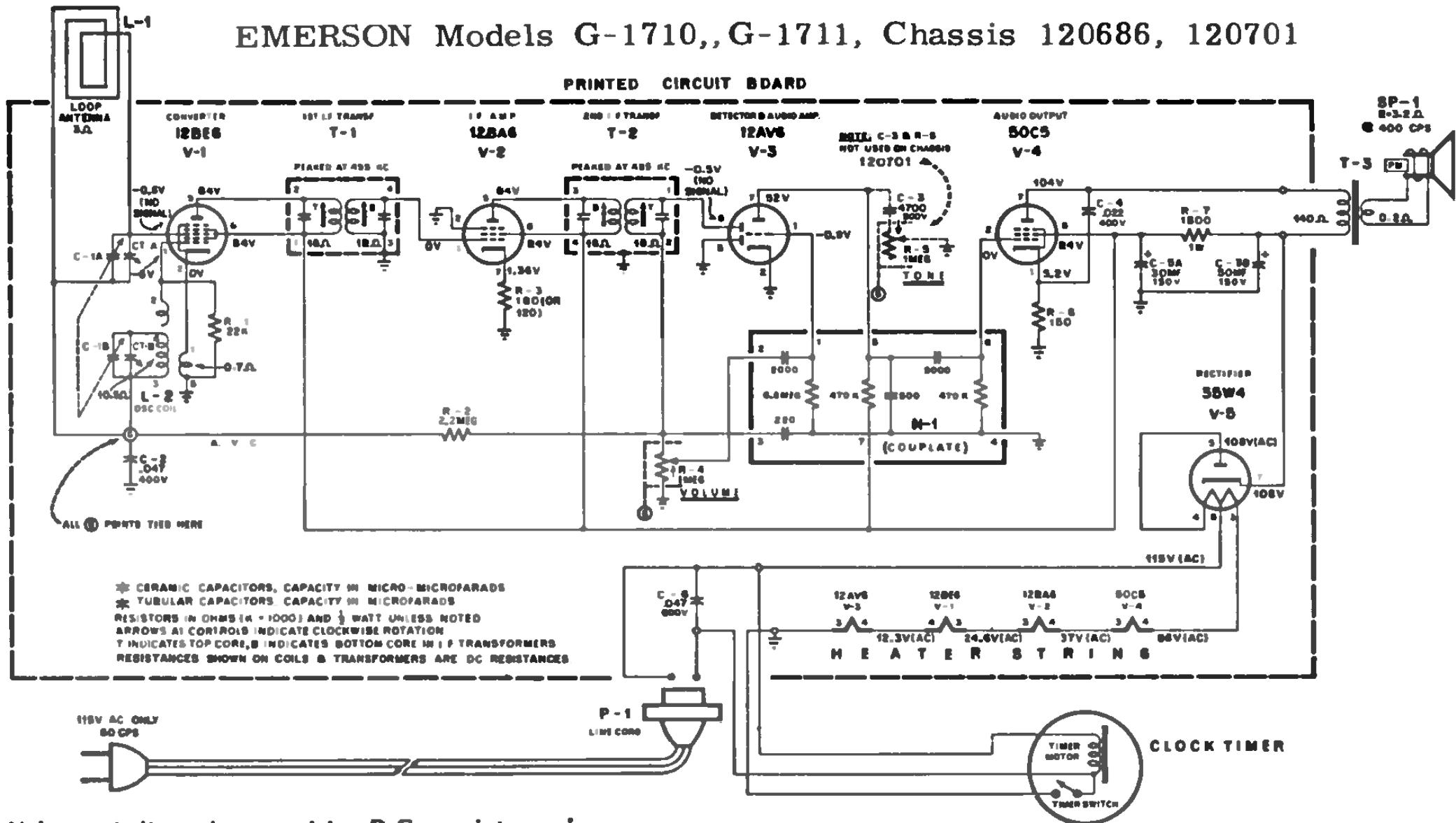
Voltages indicated are positive D.C., resistance in ohms unless otherwise indicated.
