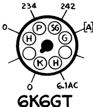
VOLTAGE MEASURED WITH 1000 OHM PER VOLT VOLTMETER BETWEEN SOCKET TERMINALS AND CHASSIS
