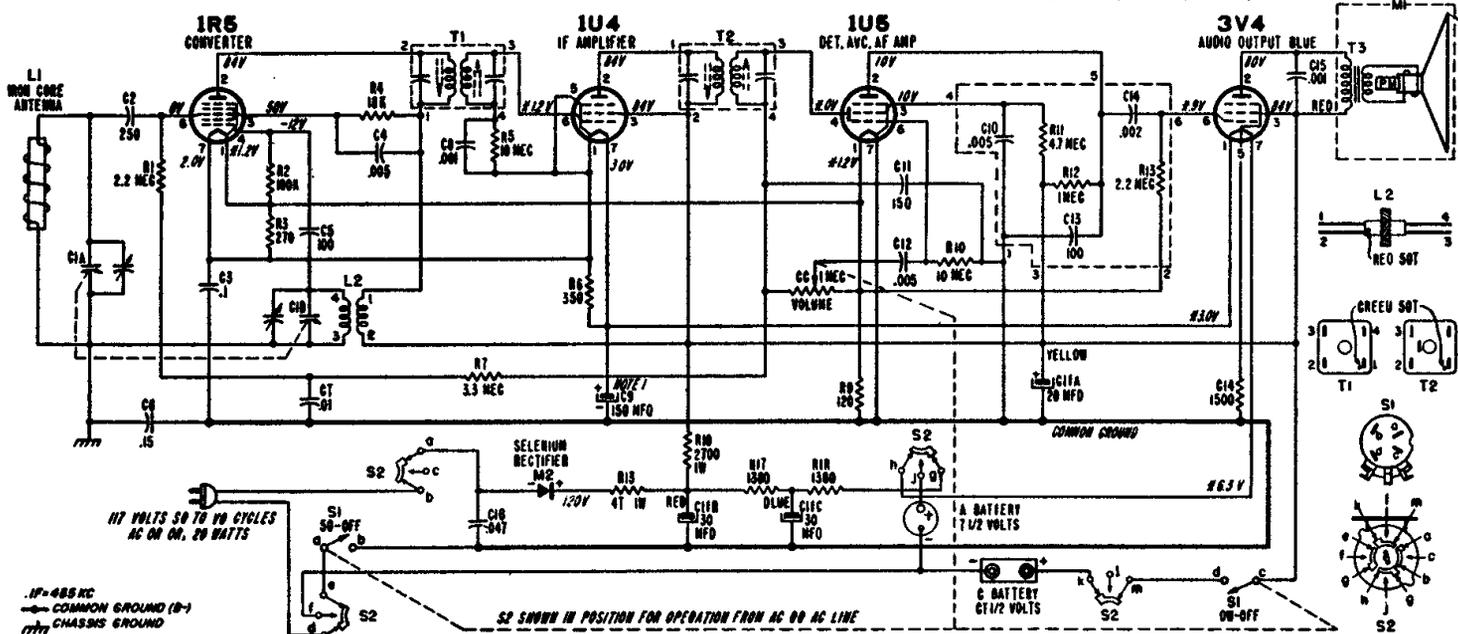
NOTE 1: C9 MAY BE PART OF C12. IF C9 IS SEPARATE, THE 100 MFD SECTION OF C12 (GREEN LEAD) MUST BE CONNECTED TO COMMON GROUND
