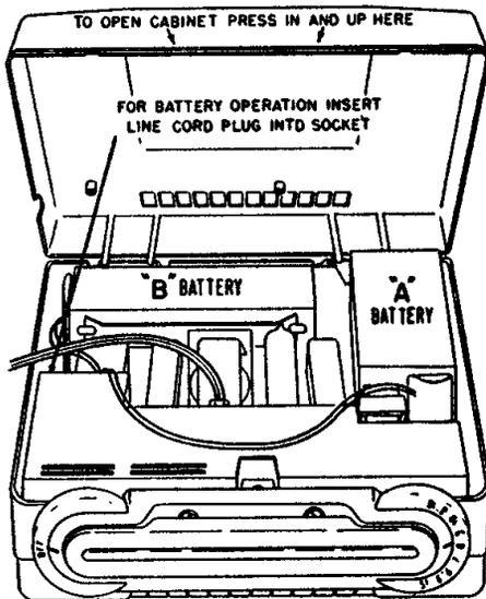
Disconnect the AC line cord from the wall outlet. Squeeze the handle support springs together near the escutcheon to remove the plastic handle. Remove the two escutcheon mounting screws. Remove the "Off-Volume" and "Tuning" knobs. Now open the cabinet (see illustration at left). Loosen the speaker mounting clips, rotate them away from the speaker, and carefully lift the chassis and batteries out of the cabinet.
