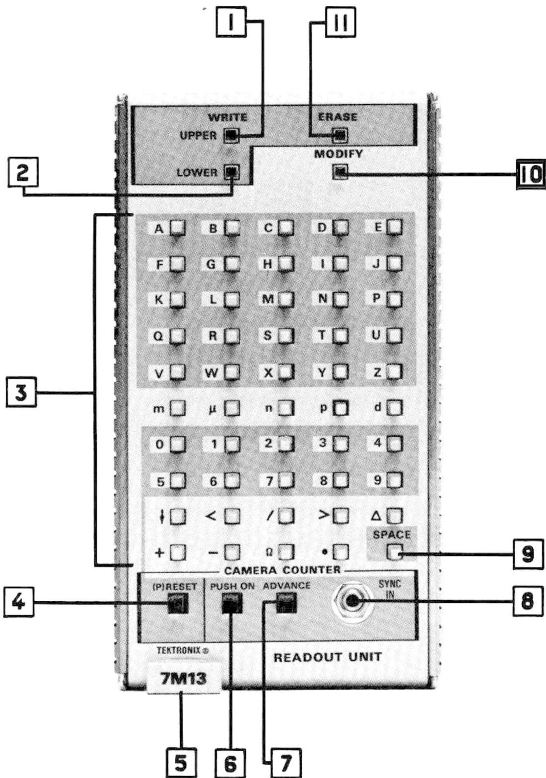
Fig. 1-2. 7M13 Controls and Connectors.
