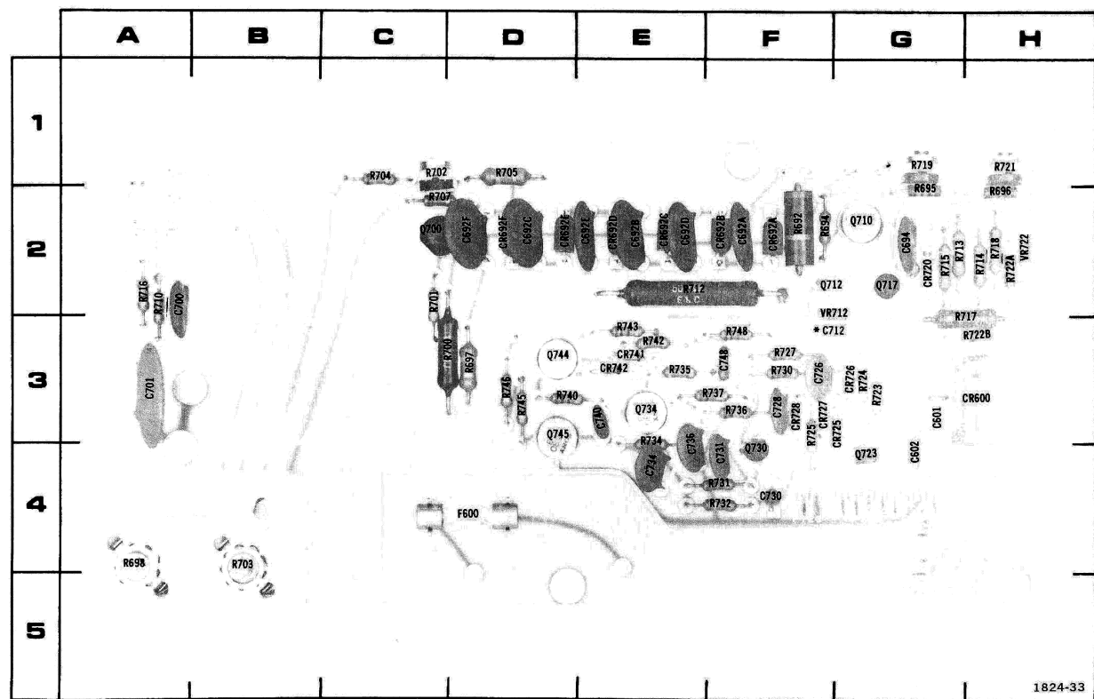
Figure 7-14B. A6-HV & Unblanking circuit board (SN 300000-300650).
