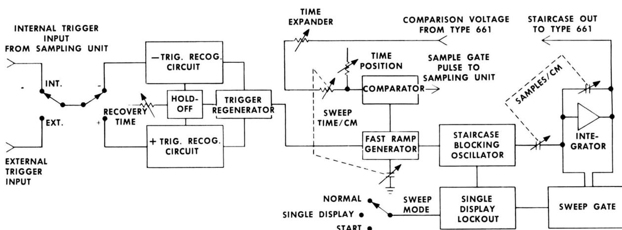
Fig. 3-1. Type 5T1A Simplified block diagram.
