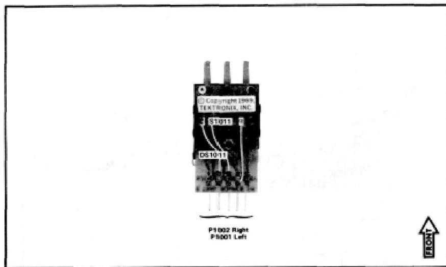
Fig. 8-21. A17 - B Trigger Source Switch circuit board.
