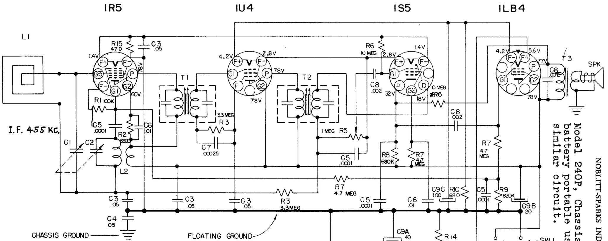
VOLTAGE MEASUREMENTS ARE MADE TO FLOATING GROUND WITH AN ELECTRONIC VOLTMETER, WITH A LINE VOLTAGE OF 117 VOLTS AC AND NO SIGNAL.
