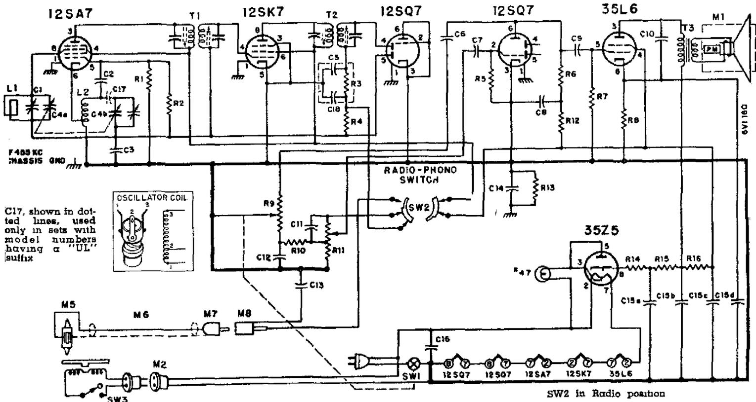
C17, shown in dotted lines, used only in sets with model numbers having a "UL" suffix
