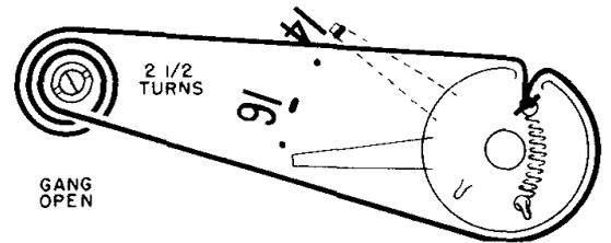
Solid lines show dial stringing and pointer position with tuning gang open. Dashed lines show pointer position (1400 KC) when tuning gang is tuned to a generator signal.
