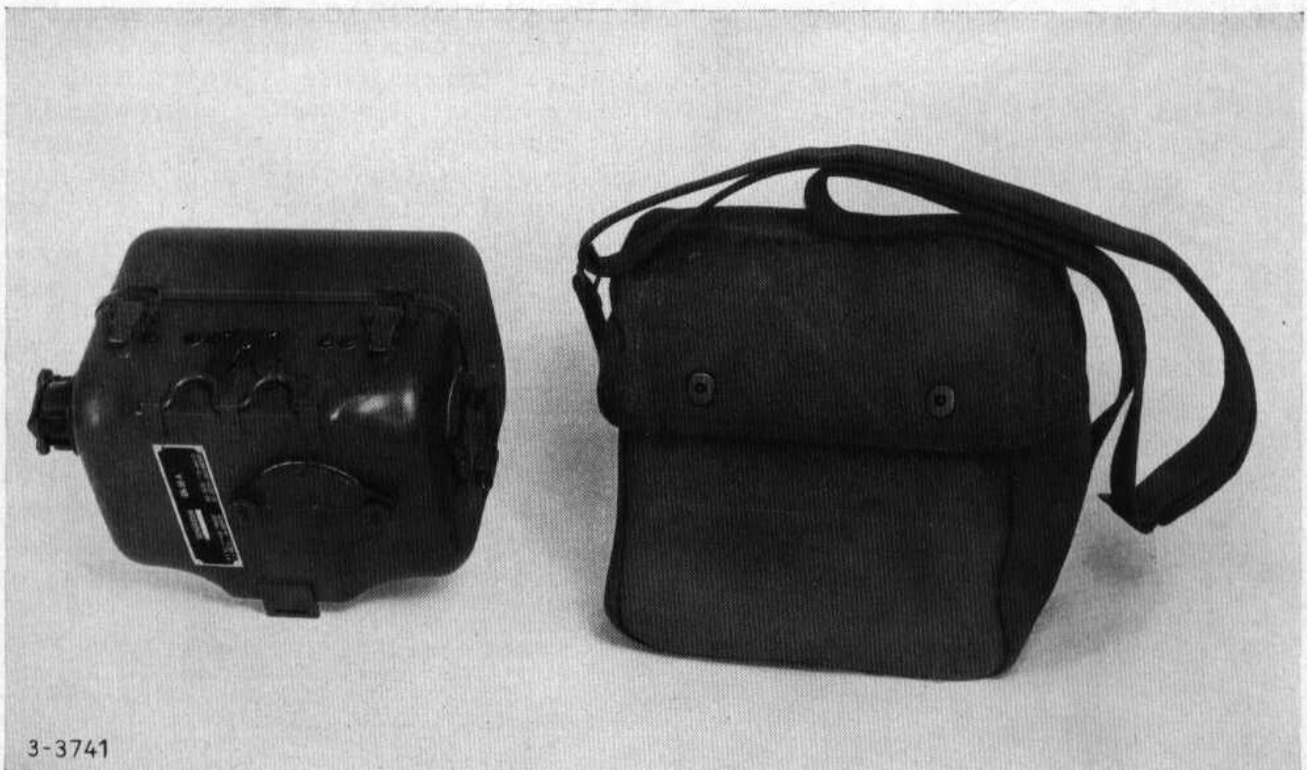
Figure 4. Generator GN-58-A-GY and Bag BG-175-GY.
