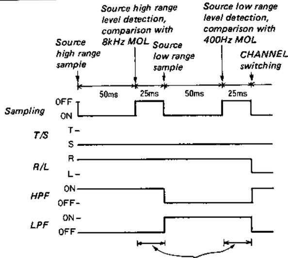
Becomes 225mS when source signal level goes over MOL value and attenuates REC LEVEL.
