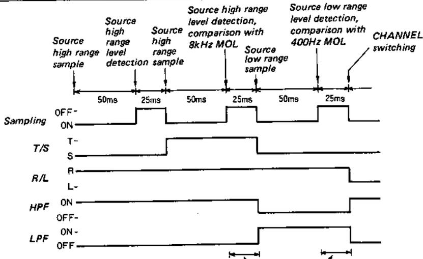
Becomes 225mS when source signal level goes over MOL value and attenuates REC LEVEL.
