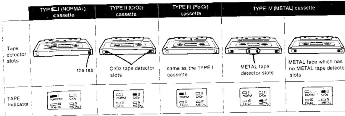
As shown in the above illustration, TYPE I, II and IV cassette tapes will be detected automatically.
