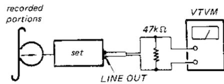
Adjust C166 (L-CH) and C266 (R-CH) so that the LINE OUT level of 333Hz signal is 0dB relative to that of 10kHz.
