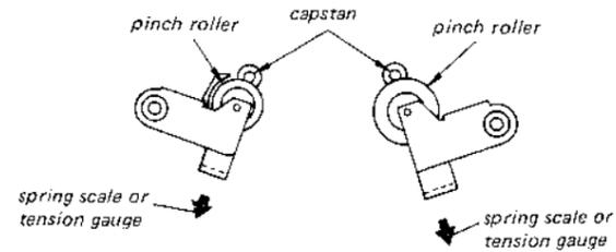
pinch roller clearance adjustment
