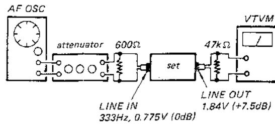
1. Set REC LEVEL for +7.5dB LINE OUT level.
