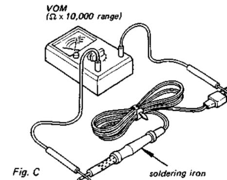
3. Equalize any potential difference between the clothes, the tools in use, the work bench, the set being worked on, and the packaged IC by touching them all in succession with the hands or a conductive wire or tool.
