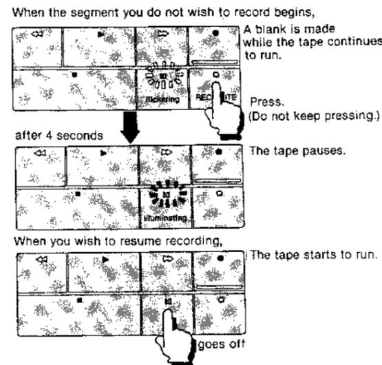
**To insert a blank less than four seconds long**
