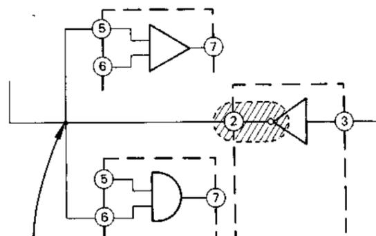
If this line is grounded, or touches B+ or B- bus . . . , the output stage of this IC will be destroyed.
