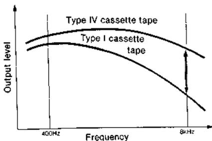
The TC-FX1010 stores in its memory the standard MOL of each of the four types of tape in the high-frequency range and low-frequency range. During recording, the input signals are divided into high- or low-frequency range and their level is compared with the memorized MOL. If their level exceeds the MOL, the automatic attenuator lowers the recording level. After the recording level has been lowered, it does not return to the original level.
