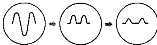
Fig. 4-7-4 Output Wave Forms when thermal protection circuit is actuated
