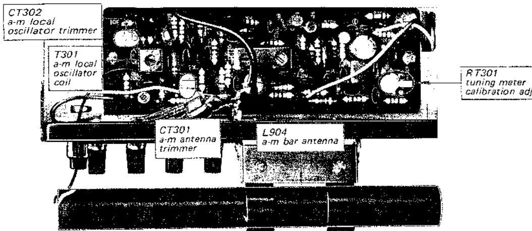
Fig. 3-14. Adjustment parts location
