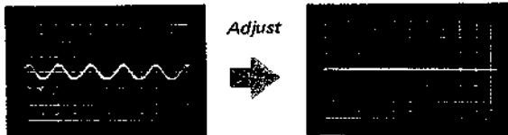
Fig. 3-6. Fm discriminator alignment output response
