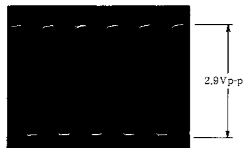
5.824 MHz master clock (Pin ⑯ of IC01) Fig. 6.
