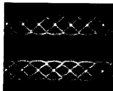
Eye pattern (Pin ⑩ of IC01 up, Pin ⑪ of IC01 down) Fig. 3-1.
