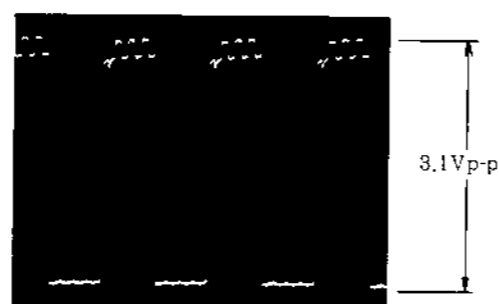
728 kHz bit clock (Pin ⑭ of IC01)
