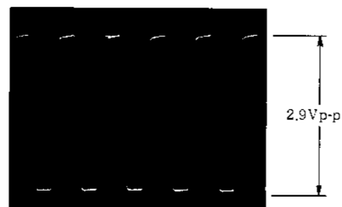
5.824 MHz master clock (Pin ⑬ of IC01)
