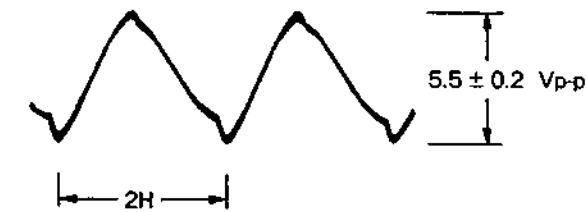
Fig. 2. SECAM ACK adjustment
