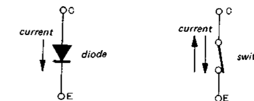
Equivalent circuit of general NPN type transistors
