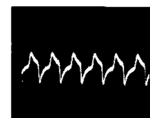
㉖ IC362 ①pin, IC502 ①,⑥pin (XIN) 3.8Vp-p, 40ns
