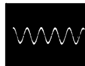
㉓ IC307 ⑥pin (XT3O) 2.9Vp-p, 0.2μs
