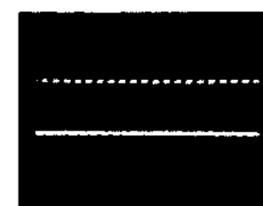
㉕ IC362 ⑥,⑤pin (DATAL, DATAR) 5Vp-p
