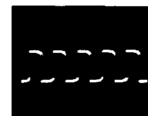
㉔ IC307 ④pin (PLCO) 4.8Vp-p, 0.18ms
