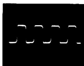
⑲ IC307 ④pin, IC359 ⑬pin (XBCK) 6.4Vp-p, 0.48μs
