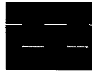
㉔ IC363 ②pin, IC601 ③pin (LRCK) 5.3Vp-p, 0.5μs
