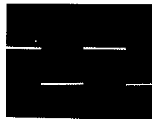
㉘ IC307 ③pin, IC311 ⑩pin (SWP) PLAY mode 5.2Vp-p, 50ms
