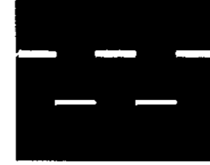
㉑ IC307 ㉑pin 6Vp-p, 0.1μs
