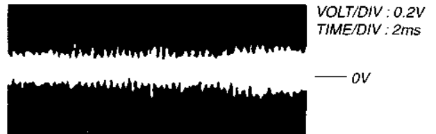
high tracking gain (high fundamental wave than for low gain)
