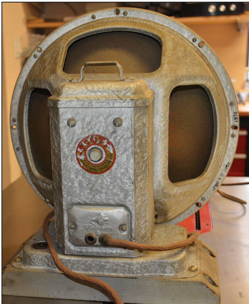
15 inch Magnavox speaker containing the crossover network for the tweeters.
