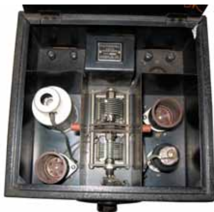
National SW-3 Receiver - Made in the early 1930s, this was a simple regenerative receiver. It used three tubes: 58, 58, 56. Originally came with three sets of coils for different bands. Arnold Corwin, Memphis, TN
