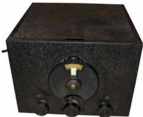
National SW-3 Receiver - Made in the early 1930s, this was a simple regenerative receiver. It used three tubes: 58, 58, 56. Originally came with three sets of coils for different bands. Arnold Corwin, Memphis, TN
