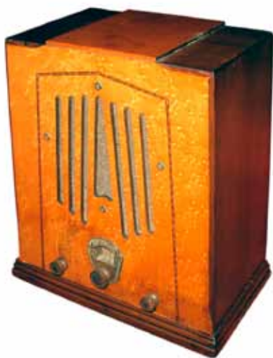
Silvertone Model 1724 Radio - Manufactured in 1934 by Sears, his TRF set originally sold for $22.95. The four tubes are: 78 RF, 77 detector, 43 output, and 25Z5 rectifier. Peter Dieguez, Roslyn, NY
