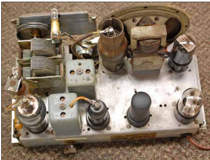
Here's the completed chassis cleaned up and ready for alignment.
