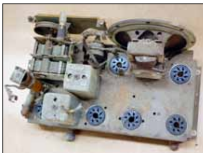
Here's another view of the chassis showing a heavy incrustation of rust and dirt.
