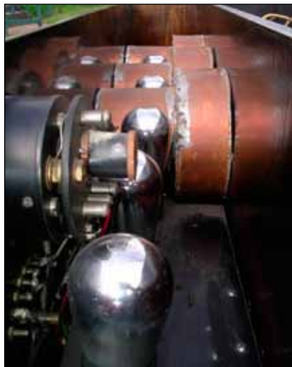
Inside view showing the copper shielding and primitive soldering.
