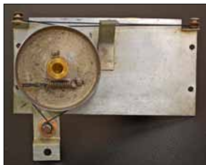
This is the dial mechanism from the back after cleaning and re-stringing.
