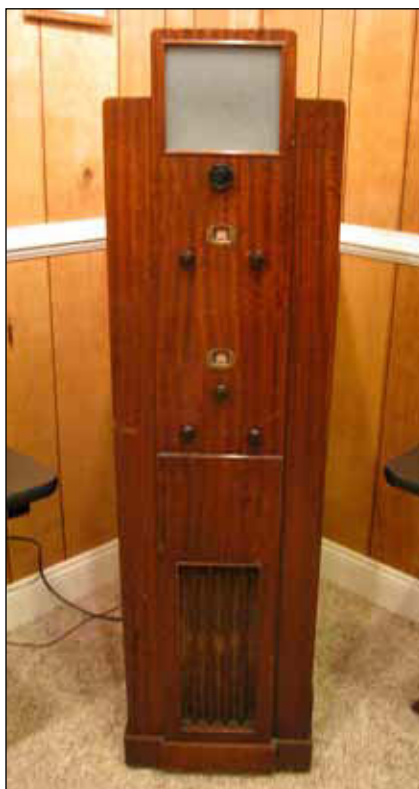
A handsome example of the 1931 Western Empire State 45 line disk receiver.
