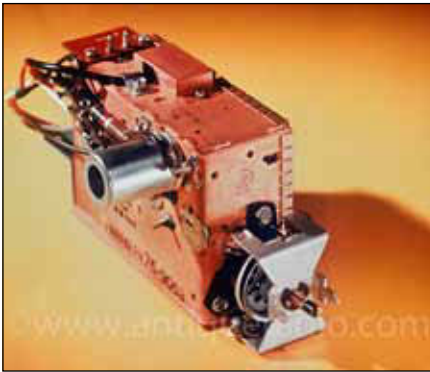
UHF Tuner – Close up of the optional new UHF frequency tuner.
