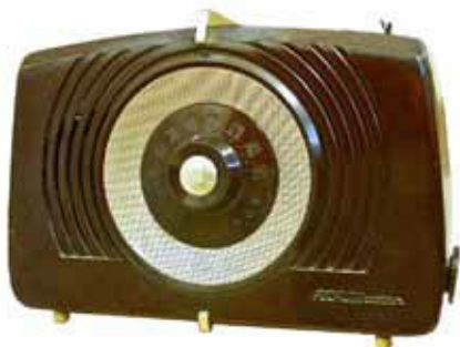
WRL model 666 VFO – This is a 6 meter VFO that uses three tubes: 6AU6, 6CB6, and 0A2. Covers 50 mc to 54 mc with an output at 8 mc. Steve Starkes, Lexington, KY
