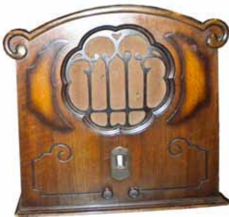
Baldwin model 70 radio – This is really a console radio whose legs were removed at some time in the past. Large radio with 12-inch speaker and seven tubes. Manufactured in 1930. Mike Katz, Seaford, NY
