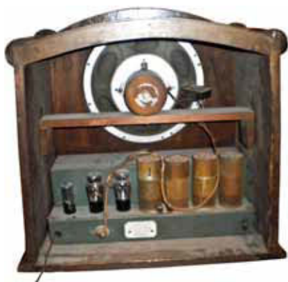
Baldwin model 70 radio – This is really a console radio whose legs were removed at some time in the past. Large radio with 12-inch speaker and seven tubes. Manufactured in 1930. Mike Katz, Seaford, NY
