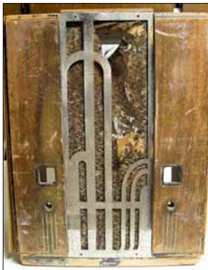
The front view of cabinet before any reconstruction and refinishing also shows how much work was ahead; note the missing bottom and destroyed grille cloth. Luckily, all three bezel pieces were in good condition and polished up nicely.
