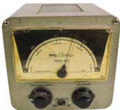
WRL model 666 VFO – This is a 6 meter VFO that uses three tubes: 6AU6, 6CB6, and 0A2. Covers 50 mc to 54 mc with an output at 8 mc. Steve Starkes, Lexington, KY
