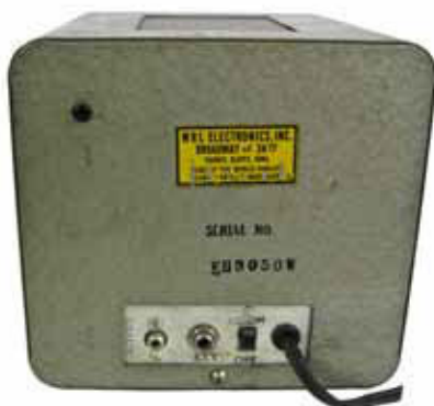
WRL model 666 VFO – This is a 6 meter VFO that uses three tubes: 6AU6, 6CB6, and 0A2. Covers 50 mc to 54 mc with an output at 8 mc. Steve Starkes, Lexington, KY
