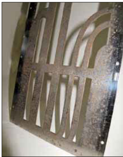
The chrome front grille removed from the cabinet and before re-chroming. Refinishing this made a huge difference in the end result.
