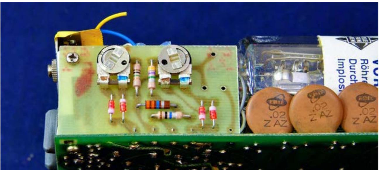
*As an aside, note the extremely high value resistors, of up to 33M $\Omega$ . Even higher values are employed on the main board.*
