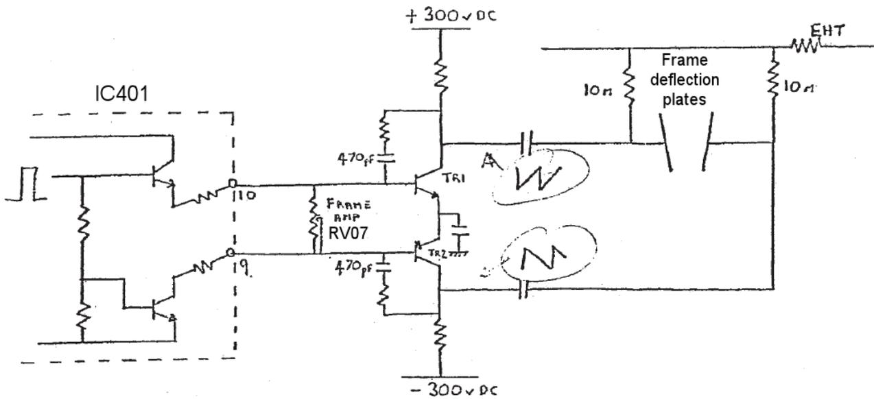
During frame flyback transistors T52 and T50 are turned on. This causes the transistors TR1 and TR2 to turn on and eventually saturate.
