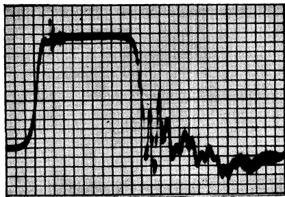
FIG. 4-5.—Voltage pulse at the grid of a 715B tube obtained from a regenerative driver using an 829 tube. Sweep speed: 10 div. per \mu\text{sec} ; pulse amplitude: 1000 volts.
