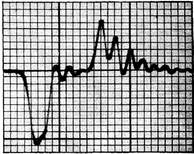
(f) Time derivative of (c) observed with long leads and mismatched cable.
