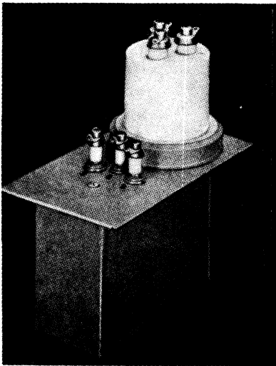
FIG. 15-36.—An airborne 250-kw 0.5- to 5.0-sec pulse transformer with a filament transformer enclosed in the high-voltage porcelain solder-seal bushing.
