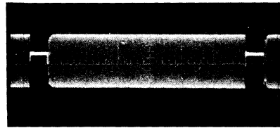
Fig. 19(b) - CA3070 terminal No. 2, 3.5 V_{p-p} oscillator output; one horizontal line, (gated off during burst).
