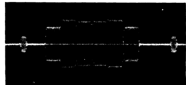
Fig. 24(a) - CA3072 - terminal No. 3 or 4, chroma input signal, 220 mV p-p , one horizontal line
