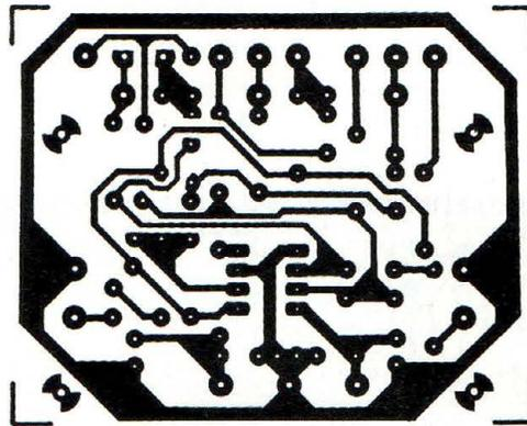
Fig.4 Reproduction du circuit imprimé version mono.
