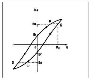
In the circuits controlled by a triac, opening occurs when the current is at zero. The induction thus has a remanent value Br, corresponding to H = 0 (*figure 5*).
