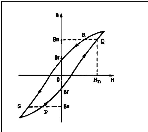
In the circuits controlled by a triac, opening occurs when the current is at zero. The induction thus has a remanent value  $B_r$ , corresponding to  $H = 0$  (figure 5).
