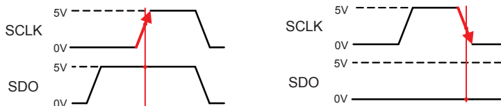
Figure 70: SPI SCLK critical edge
