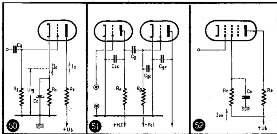
$$K = \frac{\mu R_a}{R_1 + R_a} = \frac{\mu}{1 + \frac{R_1}{R_a}} = S_a R_a. \quad (143)$$
