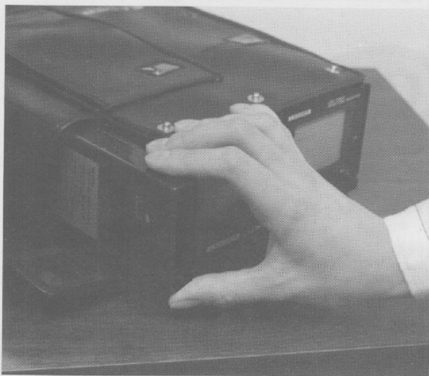
Figure 2-5. Installing the NP-1 battery
