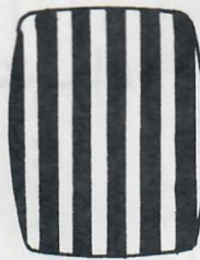
FIG. 3. HORIZONTAL BARS PRODUCED BY 400 CPS MODULATION ON SCREEN OF TV RECEIVER
