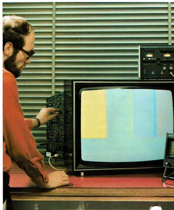
The "DEM" pattern facilitates quick and accurate alignment of the delay line circuitry.
