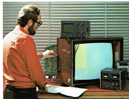
Delay line and demodulators correctly adjusted.
