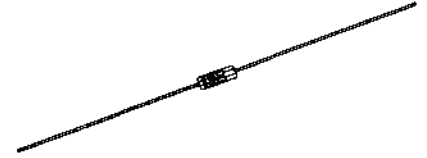
Double Heatsink Diode (DHD) IN4305
