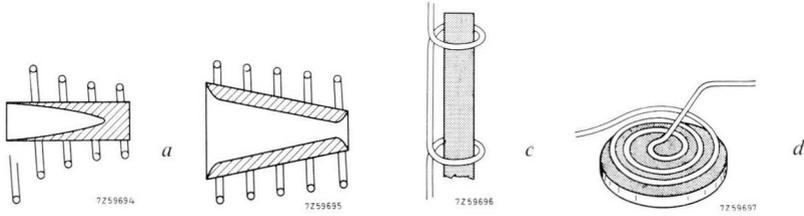
Fig. 6.10. (a). Straight cylindrical work-piece with defined temperature gradient along its axis.
