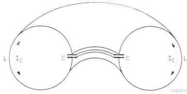
Fig. 5.24. Section of toroidal cavity with ideal inductive path length.
