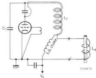
Fig. 5.38. Schematic of generator circuit where the work coil is a part of the tank coil.
