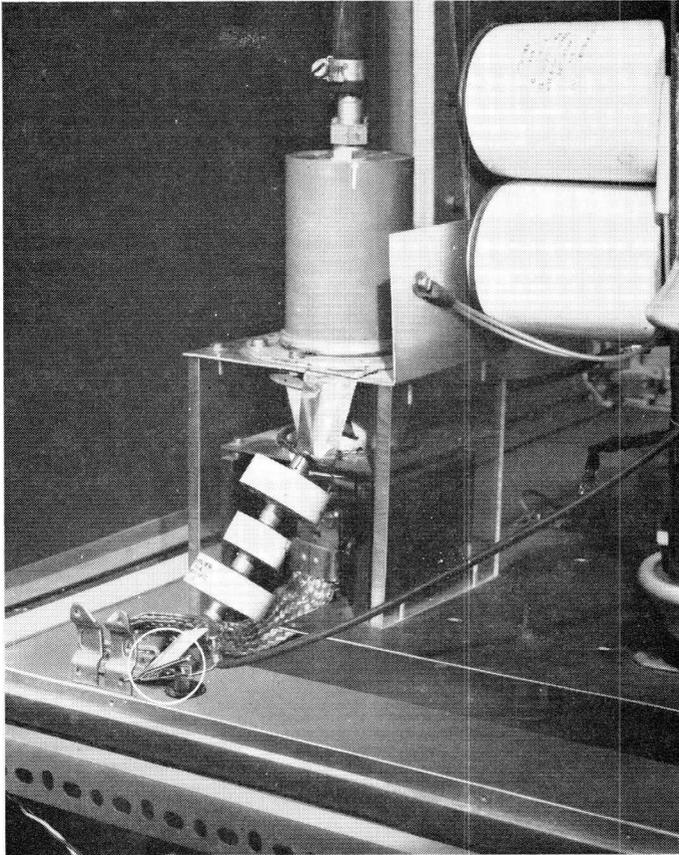
*Fig. 7.4. Capacitive divider in position. The monitoring leads are shown inside the white circle in the lower left hand corner.*
