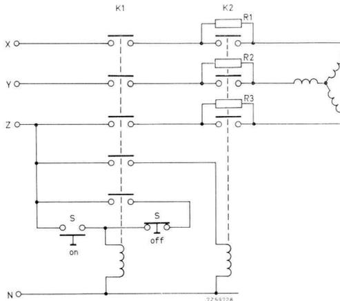
Fig. 4.11. Diagram of three-phase step switch.  $S$  is the initiating switch and  $R_{1,2,3}$  the series resistors that are short-circuited by  $K_2$  when  $K_1$  has completed its function.
