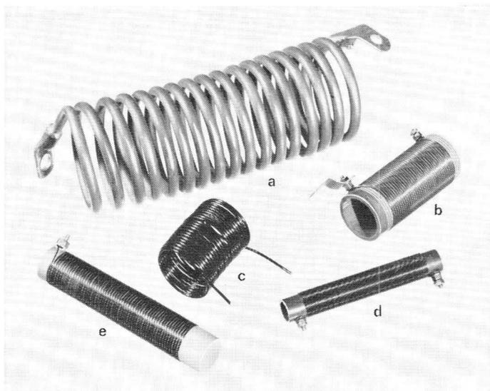
Fig. 5.36. Various types of filtering chokes that are normally used in their  $\lambda/4$  mode. (a) A 27 MHz filament choke for 140 A filament current of self supporting construction. (b) A 27 MHz choke on a threaded Paxolin former. (c) A 40 MHz self supporting enamelled wire choke. (d) A broadband 27 MHz choke with a high length to diameter ratio. (e) A 40 MHz choke wound on a Teflon former.
