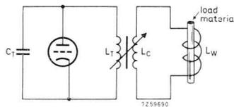
Fig. 6.6. Transformer-coupled work coil. Optimum results will be obtained if the load coupling inductor  $L_C$  is as near as possible to the effective inductance value of  $L_W$ , i.e. when the work-piece is inserted.
