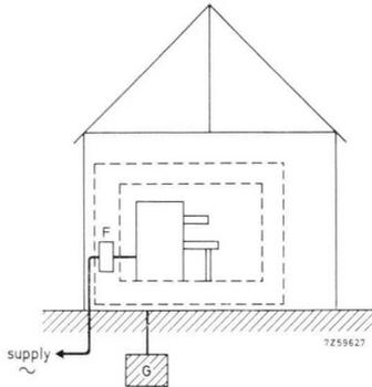
*Fig. 4.5. Sketch of double-screened work room with filter (F) in mains supply and adequate earthing (G). Metallic sections of the building structure should not be relied upon to serve as screening or earthing points because their resistance and reactance at high frequencies can be appreciable.*
