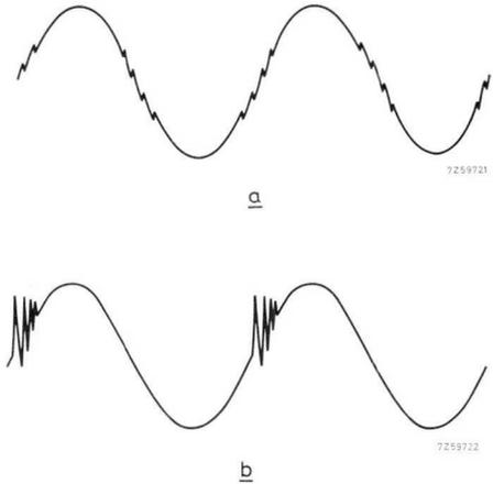
*Fig. 7.6. Tracings of parasitic high frequency envelopes on a fundamental waveform.*
