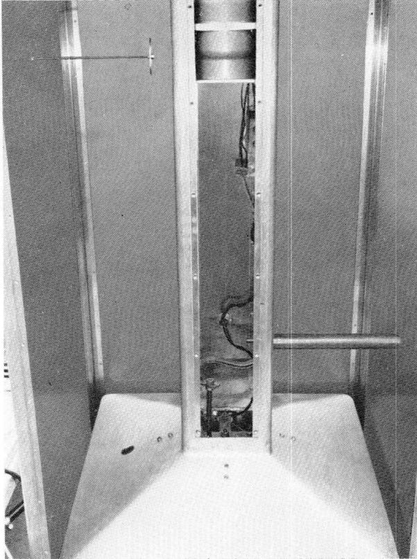
*Fig. 8.14. Generator section of line, and tank capacitor box. The 140 MHz mode absorption circuit can be seen at the top left, and the tube between the line-inner and outer can be seen at the bottom right. The tube carries supply cables for the filament, the grid bias, and mains for the coaxial air blower. Part of the blower is visible at the top, inside the line-inner.*
