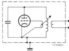
*Fig. 5.46. Schematic diagram of oscillator where all connections at nominal earth potential are returned to a small sub-chassis.*
