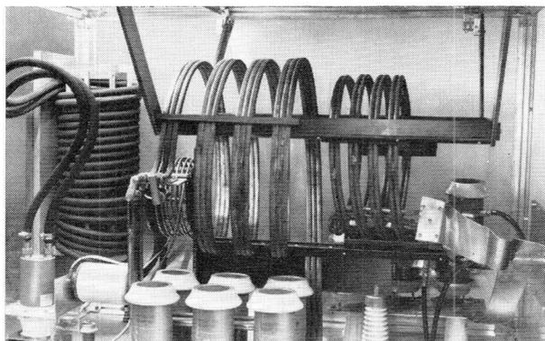
*Fig. 8.4. A detailed internal view showing typical positions of grid, tank and coupling coils.*
