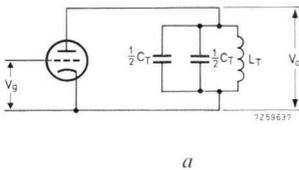
Fig. 5.5. Tube and anode tuned circuit as commonly drawn, disregarding stray reactances. A composite tank circuit capacitor has been assumed.
