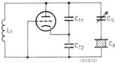
Fig. 6.15. The same directly coupled circuit as shown in Fig. 6.14 but adapted for plastic welding by using a separate and possibly variable capacitor  $C_s$  in series with the welding electrodes.
