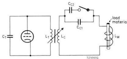
Fig. 6.8. Tuned load coupling transformer.
