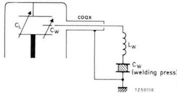
Fig. 6.22. Diagram of half-wave line load section used for plastic welding. The voltage across  $C_L$ , and  $C_L$  itself can be made large.  $C_W$  represented by the capacitive coupling probe, can be relatively small thus causing little change of the effective line and loading capacitance. Consequently, the resulting changes of operating frequency are quite small. As in the case of the dielectric heater, the load will always look purely resistive to the tube.
