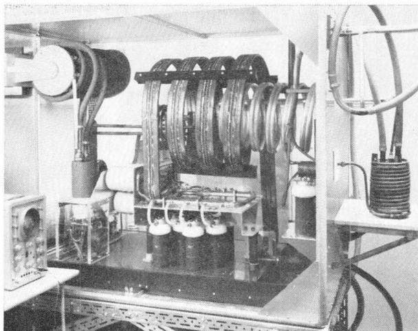
*Fig. 8.7. View of a 240 kW induction heater, constructed on similar principles as the 60 kW equipment described in the text.*
