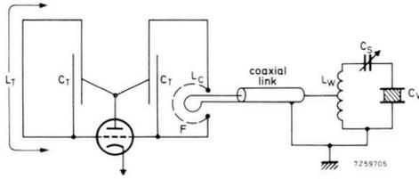
Fig. 6.19. Coaxial link coupling of cavity type generator to work coupling circuit. The frequency stability of such circuits can be very good and the load  $C_W$  can be re-matched by the capacitor  $C_S$  thus keeping the load circuit  $L_W-C_S-C_W$  in tune over the greater part of the processing cycle. Since mismatches will occur, the coaxial link should preferably be of the airspaced type to avoid irreparable voltage breakdowns.  $F$  is again the Faraday screen.
