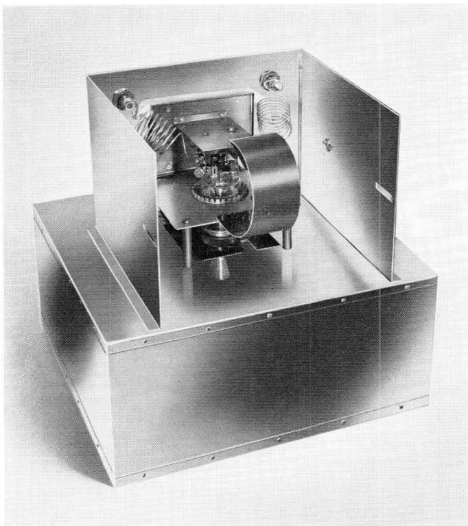
*Laboratory model of a 85 MHz, 5 kW Kolster circuit, using the TBW7/8000, suitable for dielectric heating.*
