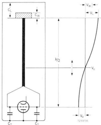
Fig. 6.21. Schematic and r.f. voltage distribution of a half-wave line generator load circuit, assuming an upward transformation from tube to load.  $V_a$  is the r.f. swing across tube and tank capacitor  $C_T$ , and  $V_L$  the voltage required across work material plus air gap.  $V_W$  is the actual material processing potential.
