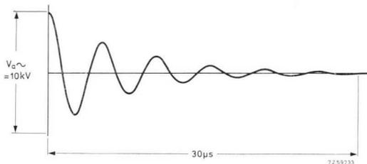
Fig. 5.49. Oscillogram of decaying r.f. anode swing of a 400 kHz oscillator after application of switching bias. The fundamental amplitude has decayed to an insignificant value within 30  $\mu$ s.
