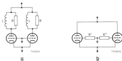
Fig. 5.2. (a) anode and (b) grid damping circuits for the suppression of inter-tube resonance in parallel operation. The resistors  $R'$  and  $R''$  need often be no more than strips of resistive material such as ferrometal alloys etc.
