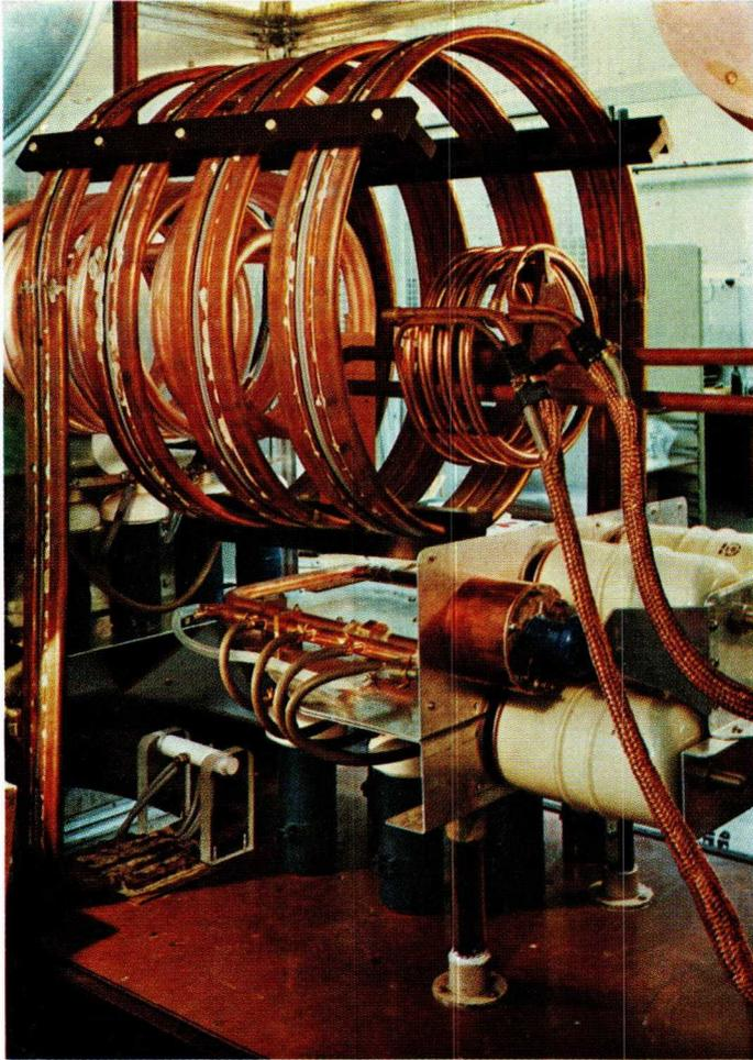
*General view of the oscillator circuit of a 240 kW, 300 kHz laboratory model induction heater (see also Ch. 8.1). The tank coil, and the grid coil with its flexible braid connections are clearly shown.*
