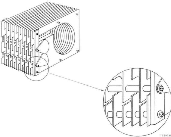
Fig. 5.19. Sectioned view of a laminated circuit.
