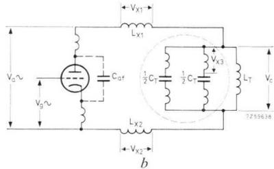
Fig. 5.6. The same circuit with some of the more obvious stray reactances inserted.
