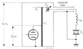
Fig. 6.20. Schematic of coaxial line generator with coaxial output and capacitive probe coupling. The tank circuit  $C_T L_T$  is formed by a capacitively loaded  $\lambda/4$  line which itself is a step-up auto-transformer.  $C_C$  is a variable capacitive probe.  $L_W$  and  $C_W$  are the inductive and capacitive components of the series-tuned load circuit.
