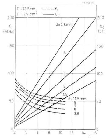
Fig. 5.20. Resonant frequency ( $f_o$ ) and circuit capacitance ( $C_c$ ) as a function of the number of plates ( $n$ ) with plate spacing ( $d$ ) as a parameter for several selected values of the cut-out diameter ( $D$ ) and the capacitive area ( $F$ ) of one resonator plate.
