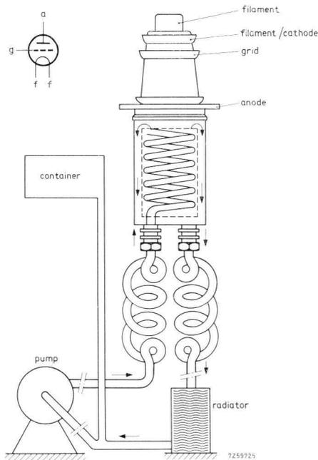
*Fig. 3.1. A typical water cooling system.*
