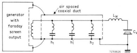
Fig. 4.4. System for removing residual harmonics between Faraday screen of generator and load position. The three traps shown in the coaxial link are in this example for two frequencies;  $h_1$  and  $h_1'$  are located at two separate high voltage points of the same harmonic and  $h_2$  at the voltage maximum of another harmonic.
