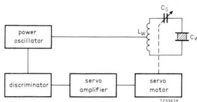
Fig. 4.6. Block diagram of load tuning with servo system. Series tuning is shown, but parallel tuning could also be used.
