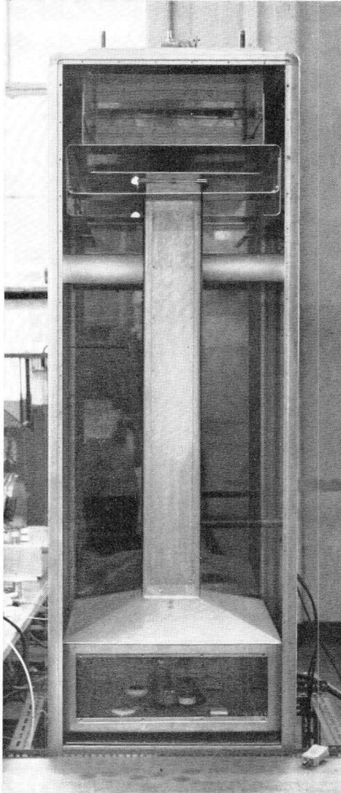
*Fig. 8.10. Overall view of 30 MHz half-wave line dielectric heater, with the front panels of the line-outer and the tank circuit capacitor box removed.*
