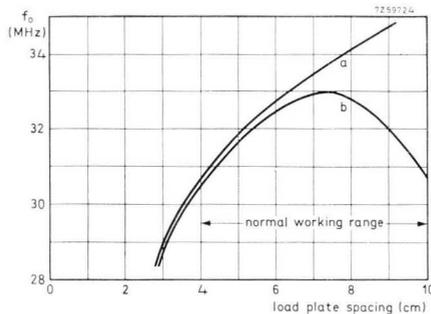
Fig. 8.16. Variation of operating frequency with spacing of the load capacitor (a) without compensation (b) with compensation by differential plates.
