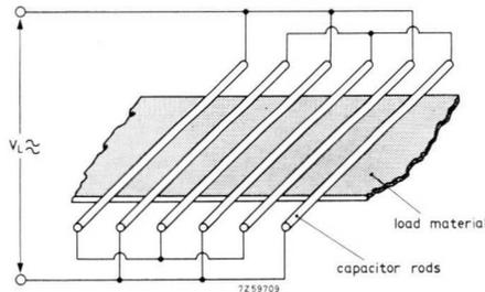
Fig. 6.25. *Stray field capacitor system with large area load underneath.*
