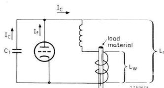
Fig. 6.4. Directly-coupled induction heater with a work coil that constitutes only part of the main tank circuit inductor.
