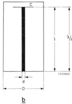
Fig. 5.29. (b). Coaxial line showing the various dimensions required for calculation.
