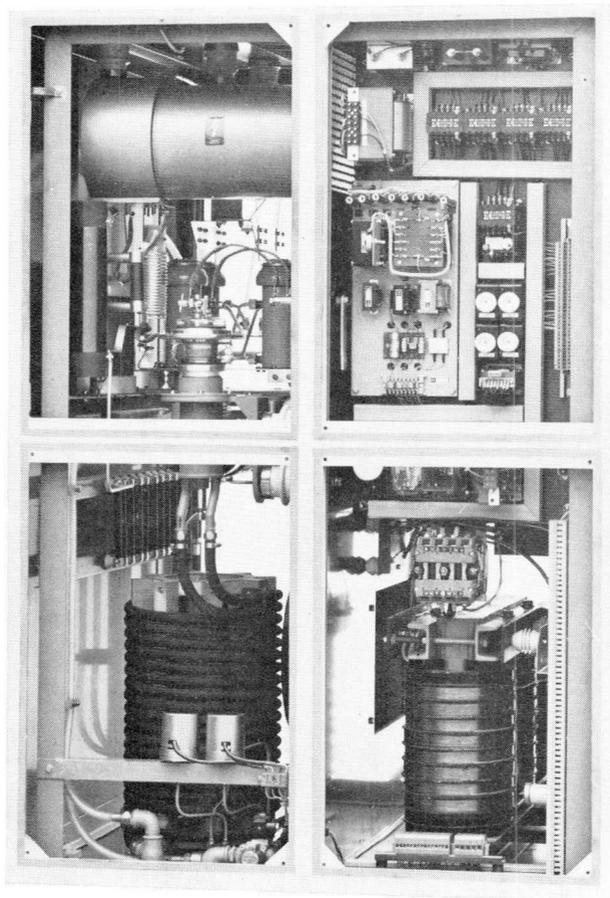
*7 kW generator (frequency 200-800 kHz) using tube type TBW6/14 (by courtesy of Fritz Hüttinger Elektronik GmbH, Freiburg, Western Germany).*
