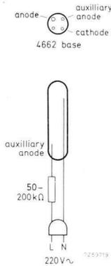
Fig. 7.2. Diagram of probe.
