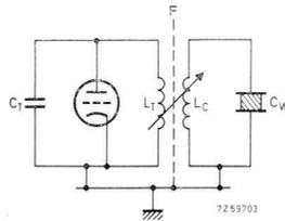
Fig. 6.17. Example of simple transformer-coupled load. For maximum power transfer the load circuit  $L_C/C_W$  should be tuned near the operating frequency of  $L_T/C_T$  at the peak of the processing cycle. The power transfer may also be varied by adjusting the coupling between  $L_T$  and  $L_C$ .  $F$  is the Faraday screen, preventing capacitive coupling between oscillator and load circuit.
