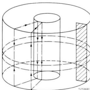
Fig. 5.44. Toroid cavity.
