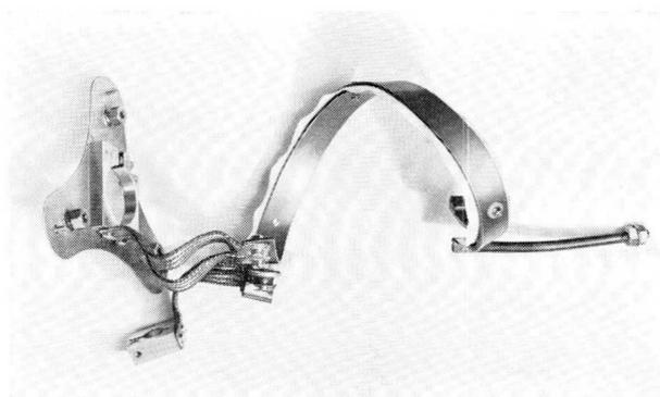
*Fig. 8.12. Grid-cathode circuit inductor with filament connectors.*
