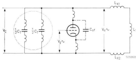
Fig. 5.7. Capacitive and inductive components, including strays, are so grouped that only the minimum of the opposing vector is effective in each composite reactance.  $L_{x1,2}$  are now part of the main tank inductor.
