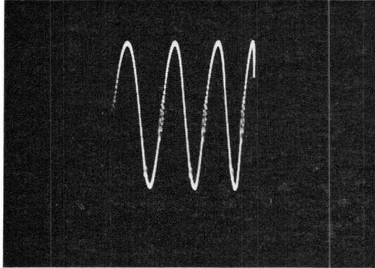
*Fig. 7.5. Oscillogram of 400 kHz waveform. The slight ripple on the waveform is due to component ringing. Since its amplitude is less than 5% of that of the fundamental it can be ignored.*
