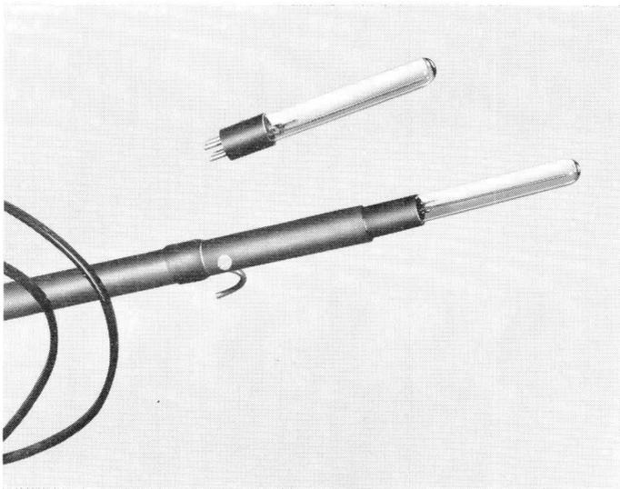
*Fig. 7.3. Neon tube shown separately and connected to its wander probe.*
