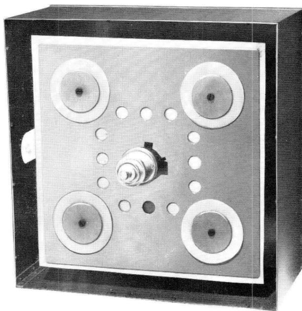
*Fig. 5.28. Kolster circuit designed for operation at 85 MHz.*
