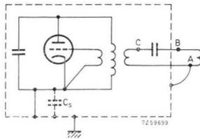
Fig. 6.13. Example of correct location of earthing points in an induction heater.
