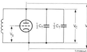
Fig. 5.8. Preferred diagram, indicating the logical component layout in a generator circuit.
