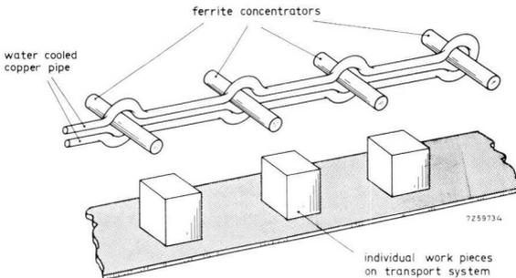
Fig. 6.12. Ferrite current concentrators. Sufficient cooling of the ferrite concentrator is ensured if it is in good thermal contact with the water cooled r.f. conductor of the load coil.
