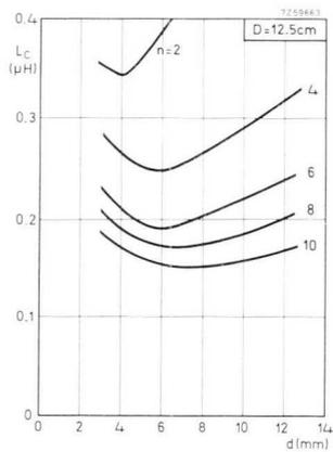
Fig. 5.21. (b). Circuit inductance ( $L_c$ ) as a function of the plate spacing ( $d$ ) with the number of plates ( $n$ ) as parameter for several selected values of the cut-out diameter ( $D$ ).
