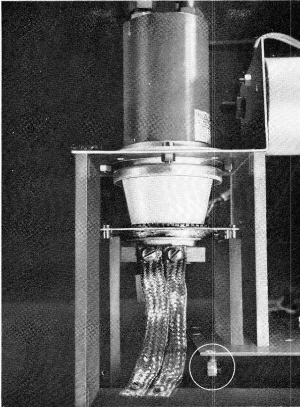
*Fig. 8.6. The YD1182 mounted in the cabinet. The earthing bolt connecting the tank capacitor plate to the chassis is visible at the bottom centre.*
