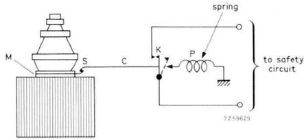
Fig. 4.8. Fuse link to tube anode. A metal band *M* is fixed around the neck of the tube and has on one side a soft solder joint, *S*. An insulated cord *C* holds contact *K* closed against spring tension of *P*. In case of overheating *S* melts and releases cord, causing *K* to go open-circuit.
