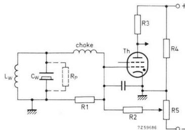
Fig. 5.50. Schematic diagram of arc suppression circuit.
