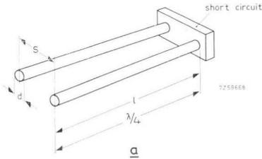
Fig. 5.29. (a). Lecher line with  $\lambda/4$  characteristic.
