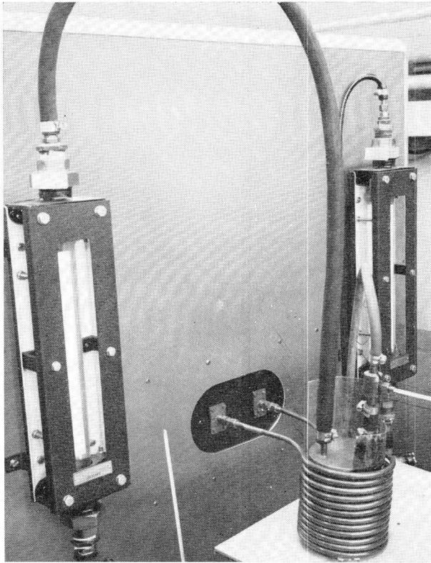
*Fig. 8.3. View showing work coil and water cooled load can with mica insulation to prevent shorting of the coil. The flow meters and thermometers used in some of the measurements are also shown.*
