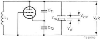
Fig. 6.14. Example of directly coupled dielectric heater where  $V_a$  is sufficiently large to equal  $V_w + V_{gap}$ . The oscillator circuit shown is a Colpitts type, but other systems could be used.
