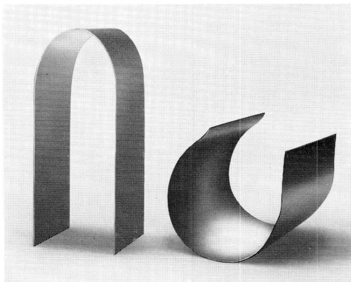
*Fig. 5.11. Examples of tank inductors of a high  $C/L$  ratio in the 27 MHz range. At this frequency and with a copper construction, the inductor loop widths must be approximately 2 cm per kilowatt of the tube output to avoid undue circuit losses.*
