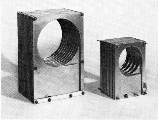
Fig. 5.22. A comparison of the laminated circuits used for 75 MHz (120 pF) and 20 MHz (560 pF).
