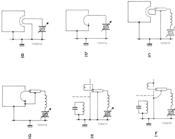
Fig. 6.29. Correct (a, c, e) and incorrect (b, d, f) load circuit and earth return connections on cavity type generators with inductive coupling.
