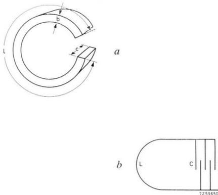
Fig. 5.16. Schematic diagram of (a) lumped circuit inductor and (b) of a lumped circuit.
