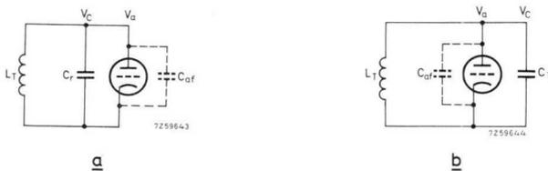
Fig. 5.10. The layouts have the following in common:  $C_{af} < C_T$ ,  $X_{C_{af}}$  high and  $X_{C_T}$  low at the parasitic frequency but:
