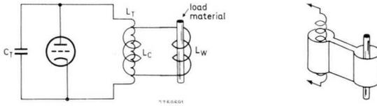
Fig. 6.7. Schematic diagram and sketch of single turn "wrap around" load coupling coil.
