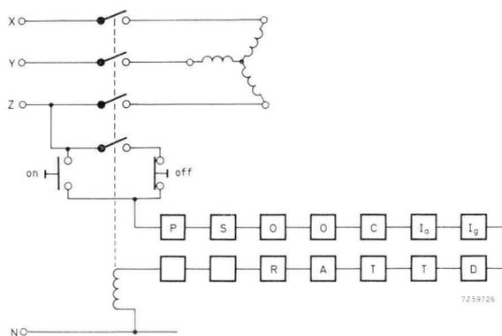
Fig. 4.7. General safety circuit with interlocks for: *P* access panels, *S* safety cover, *O* operators push-buttons, *C* cooling plant,  $I_a$  anode current,  $I_g$  grid current, *D* delay switches, *T*, process timers, *A* anode temperature sensing, *R* arc protector.
