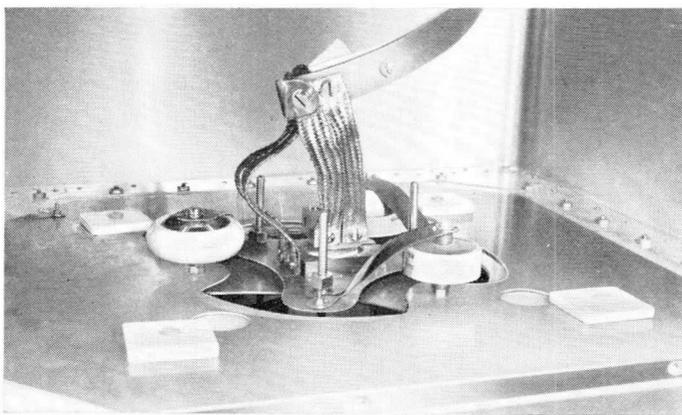
*Fig. 8.13. Grid-cathode circuit and feedback assembly. Three ceramic capacitors (total 140 pF) are grouped round the tube header and connected between filament (cathode) and grid plates. The three adjustable rods, holding the feedback ring, can be seen protruding from the collets on the filament (cathode) plate.*
