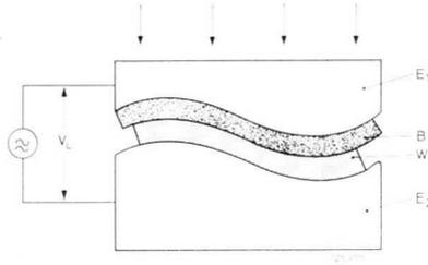
Fig. 6.27. Wood shaping electrodes.
