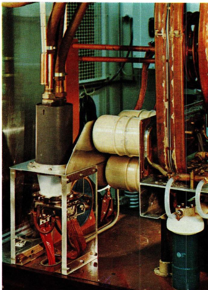
*The YD1212 of the 240 kW induction heater is shown mounted on Perspex side panels. The thermometer with which the rise in temperature of the anode cooling water is read can be seen attached to one of the water feed pipes.*
