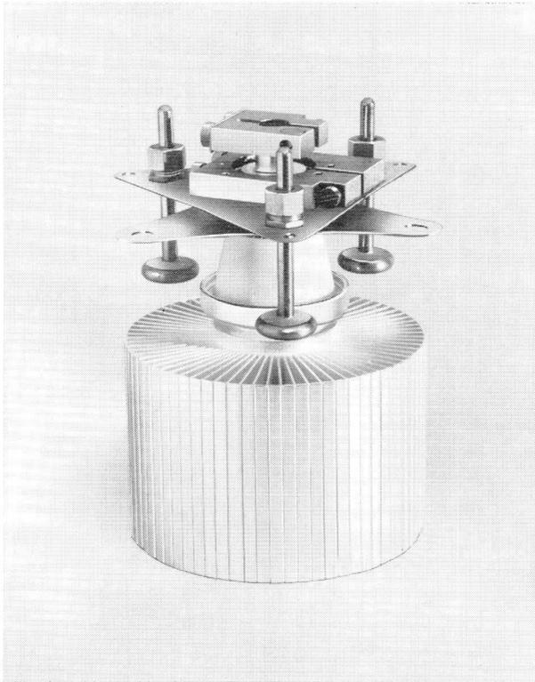
*Fig. 5.31. Grid and filament connectors and feedback probes fitted to YD1150 when used as a common grid oscillator. The necessary feedback capacitance  $C_{af}$  is formed by the probes looking at the anode cooler (or mounting flange if water cooled tubes are used).*
