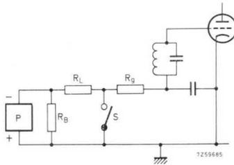
Fig. 5.48. Basic grid switching circuit.
