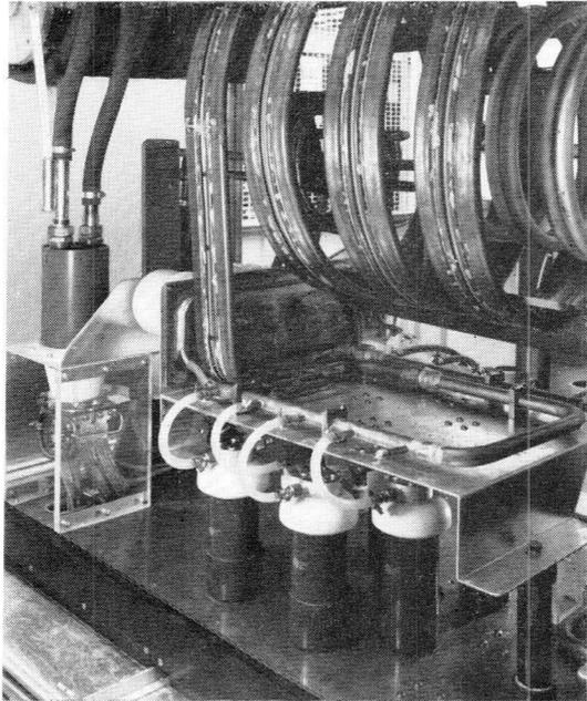
*Fig. 5.15. A general view of a coil and capacitor tank circuit. This tank circuit is used with a YD1212 in a 240 kW induction heater developed by our application engineers.*
