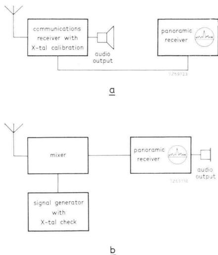
Fig. 7.7. Schematic diagram of panoramic receiver installation. Either (a) or (b) will form a testing set-up, suitable for the frequency checks outlined in the text.
