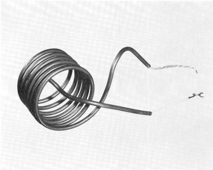
Fig. 5.37. (a). Total self decoupling of anode supply line in induction heating generator with separate load circuit. At the point of emergence from the oscillatory circuit the h.t. line is free of radio frequency and no further decoupling elements are necessary. (b) Inductor designed as feedback for a low-frequency induction heater using the self decoupling method. The Fibreglass covered grid lead is fed through the centre of the inductor thus avoiding the use of separate grid chokes.
