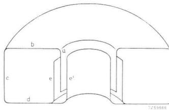
Fig. 5.25. Section through toroidal cavity tank circuit. If the area enclosed by the sides  $a$ ,  $b$ ,  $c$ ,  $d$  and  $e/e'$  approximates to a square, the value of the inductive component can be given by
