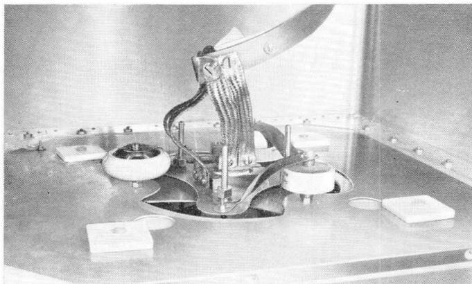
*Fig. 5.32. Grid-cathode circuit and feedback assembly. Three ceramic capacitors (total 140 pF) are grouped around the tube header and connected between filament (cathode) and grid plates. The three adjustable rods holding the feedback ring can be seen protruding from the collets on the filament (cathode) plate.*
