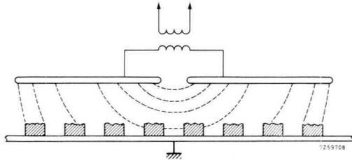
Fig. 6.24. *Balanced applicator electrodes.*
