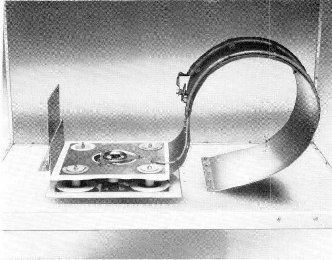
*Fig. 5.17. An example of a well integrated coil and capacitor assembly forming a 27 MHz tuned circuit. The faces of the tank capacitor are used to accommodate the respective anode and grid blocking capacitors and the tubes running along the inductor section carry the feedlines to the grid and filament voltage. This is an excellent example of the self decoupling techniques discussed in Ch. 5. The tube and the feedback components are not shown.*
