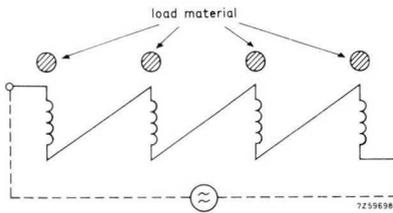
Fig. 6.11. Schematic diagram of individual load positions with series connected work coils fed from a common generator. Such a system is particularly suitable for continuous production lines involving small work-pieces.
