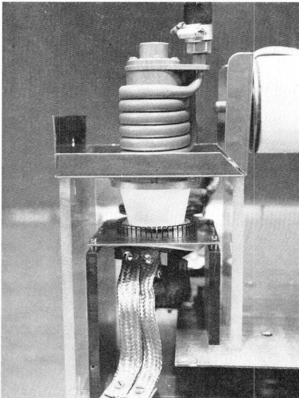
*Fig. 8.5. The YD1172 mounted in the cabinet.*
