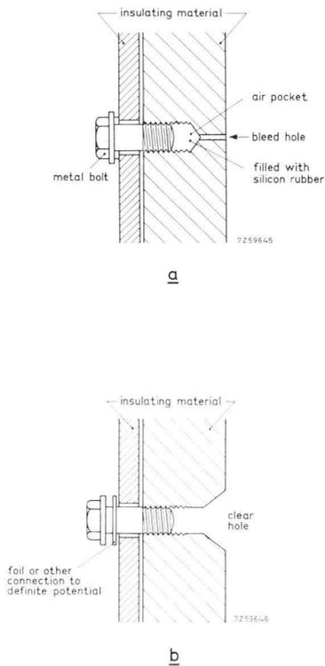
*Fig. 5.12. To avoid ionization damage the brass bolt shown should be tied to a definite potential and so dimensioned that it will fill the threaded hole completely, or alternatively the hole drilled right through the insulating material. Where requirements for mechanical strength are not so high bolts manufactured from insulating material can be used.*
