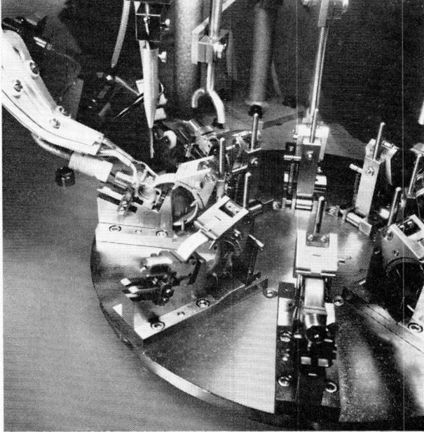
*A 6 kW r.f. generator for soldering manometer parts, using tube type TBL7/8000 (by courtesy of Himmelwerk A.G., Tübingen, Western Germany).*
