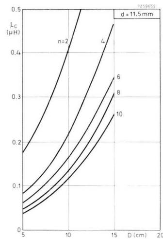
Fig. 5.21. (a). Circuit inductance ( $L_c$ ) as a function of the cut-out diameter ( $D$ ) with the number of plates ( $n$ ) as parameter for several selected values of the plate spacing ( $d$ ).
