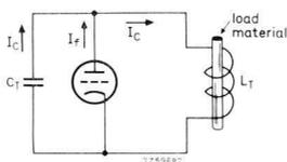
Fig. 6.3. Schematic of directly coupled induction heater where the whole of the tank circuit inductor forms the load coil. The current through this coil  $I_c = I_f \times Q_L$  where  $I_f$  is the r.m.s. value of the fundamental tube current.
