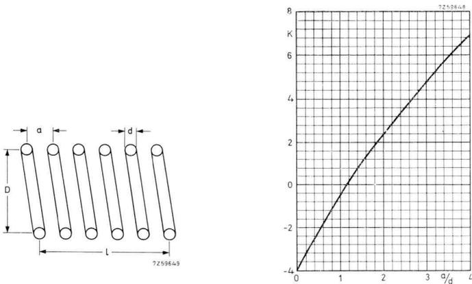
Fig. 5.14 (a). The derivation of the factor  $K$  from the coil dimensions.
