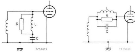
Fig. 5.43. Series and parallel tuned suppressor circuits.
