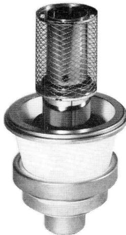
*Fig. 1.2. Mesh cathode construction.*
