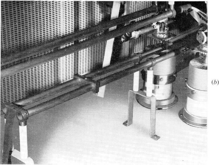
Fig. 5.4. A lecher line oscillator shown in its schematic form (a) and a practical circuit (b).
