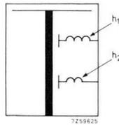
Fig. 4.3. Capacitively loaded line or Kolster circuit with harmonic absorption circuits for the frequencies  $h_1$  and  $h_2$ . Accurate resonance is obtained by trimming either the inductive or capacitive components of these circuits.
