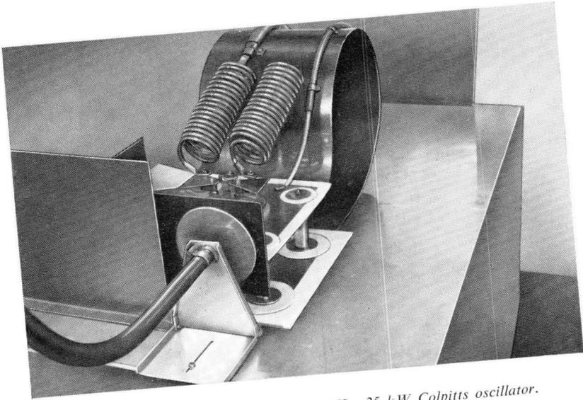
*Fig. 5.39. Self decoupling on a 27 MHz, 25 kW Colpitts oscillator.*
