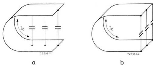
Fig. 5.9. Example of incorrect (a) and correct (b) positioning of individual capacitive components on a U-shaped strip inductor. The incorrect disposition of the capacitive components will result in a higher frequency and degraded  $Q_L$  as well as uneven current sharing through the individual capacitors.
