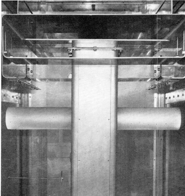
*Fig. 8.15. Load section of the half-wave line with the load position capacitor. The differential capacitive plates can be seen to be preset, adjustable in relation to the main variable plate. The horizontal polypropylene tubes can also be seen.*
