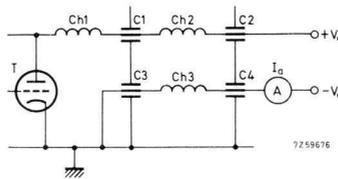
Fig. 5.41. Example of double filtering network in the h.t. supply of a generator.  $Ch_{1,2,3}$  are  $\lambda/4$  chokes or other suitable inductors.  $C_{1,2,3,4}$  are feedthrough capacitors mounted on partitioning panels. The negative supply line is also filtered and connected near the tube cathode.
