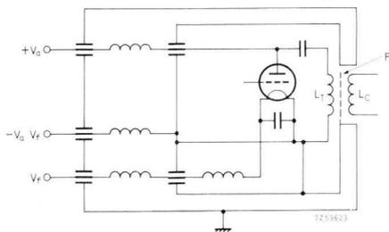
Fig. 4.1. Example of double-screened generator box with  $\pi$  filtering networks consisting of feedthrough capacitors and chokes. A Faraday screen,  $F$ , is inserted between the tank circuit coil  $L_T$  and the load circuit coupling coil  $L_C$ .
