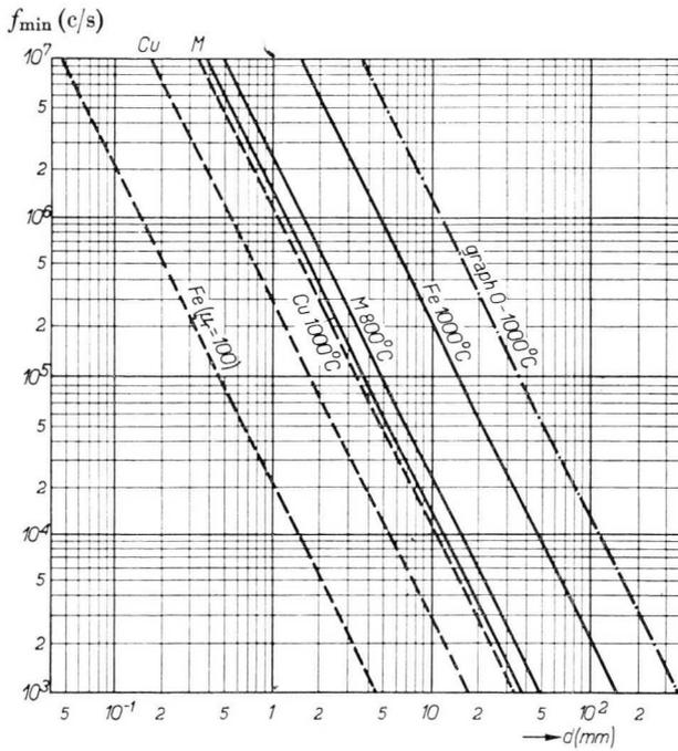
Fig. 6.1. The lowest frequency  $f_{\min}$  at which the efficiency is not unnecessarily low, as a function of the diameter  $d$  of the work-piece, for graphite (graph), iron (Fe), copper (Cu) and brass (M), at room temperature (dotted lines) and at 800-1000°C (fully drawn lines). For cold iron it has been taken that  $\mu_r = 100$ .
