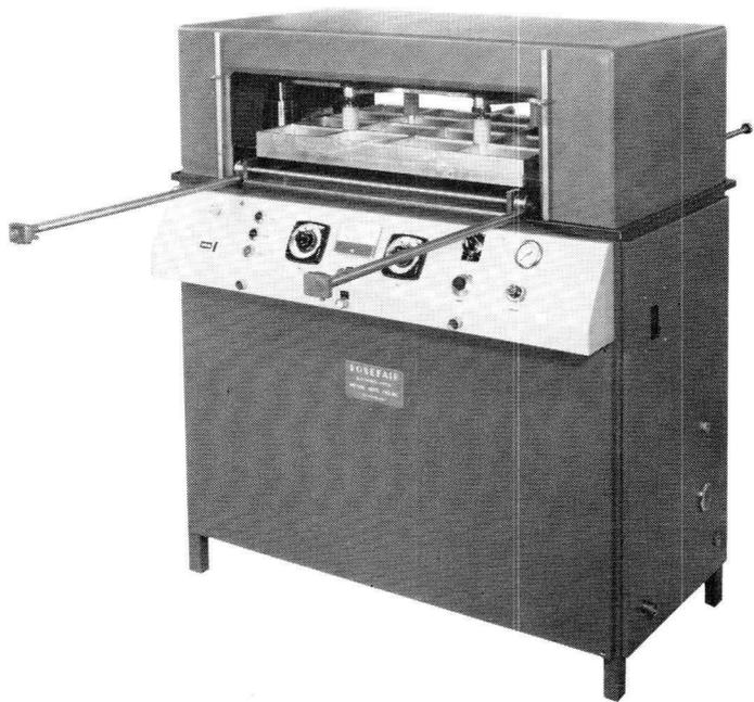
*A 7 kW plastic welder using tube type YD1160 (by courtesy of Rosefair Electronics, Watford, England).*
