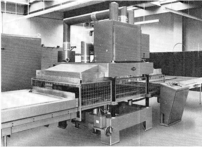
*An HF welding press (10 ton pressure) fed from a 40 kW, 27.12 MHz generator using 2 tubes TBL12/25 (by courtesy of Herfurth GmbH, Hamburg, Western Germany).*
