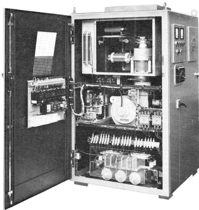
*27.12 MHz generator supplying 10 kW at the electrodes, using tube type YD1173
