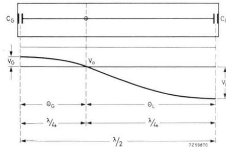
Fig. 5.30. Voltage distribution along a half-wave line with capacitively loaded ends.
