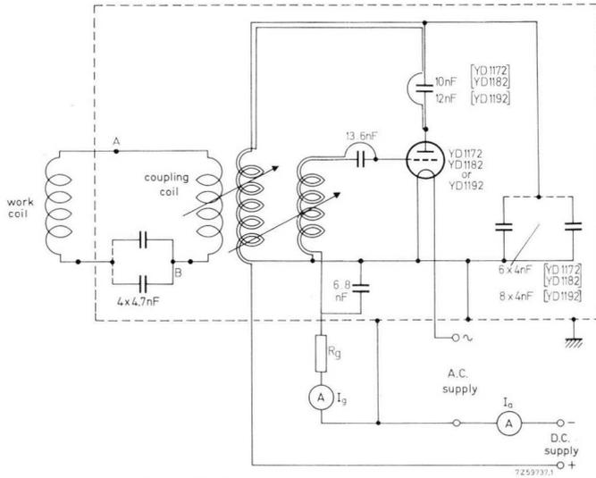
Fig. 8.1. Circuit of induction heater oscillator.
