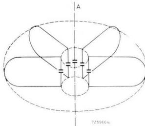
Fig. 5.23. Development of toroidal cavity by the rotation of a lumped circuit around the axis A.
