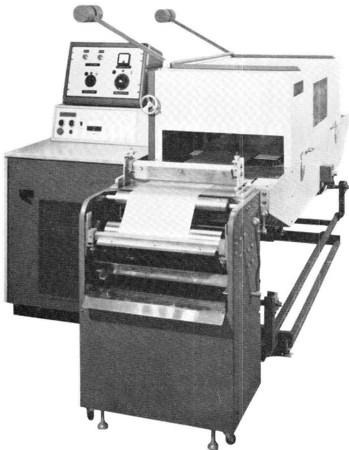
*7.5 kW, 27 MHz generator used for profile drying of paper (by courtesy of Intertherm, London, England).*
