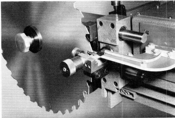
*A 2 kW generator for soldering hardened material on to saw blades, using tube type TB5/2500 (by courtesy of Himmelwerk A.G., Tübingen, Western Germany). The inductor arrangement is shown enlarged.*
