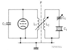
Fig. 6.18. Transformer-coupled load circuit containing a series capacitor  $C_S$  that may be used for power control purposes or the retuning of the load when the work material characteristics change during the process.
