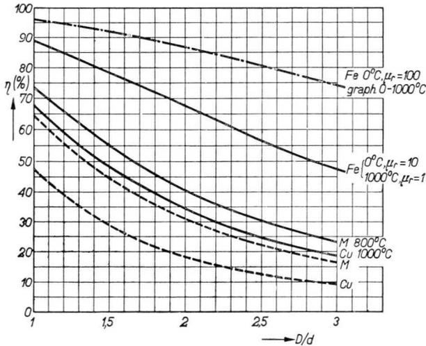
Fig. 6.2. Efficiency  $\eta$  of the work coil as a function of  $D/d$  ( $D =$  diameter of the work coil,  $d =$  diameter of the work-piece) for various materials, at  $0^\circ\text{C}$  (dotted lines) and at  $800-1000^\circ\text{C}$  (fully drawn lines). For cold iron a curve has been plotted for  $\mu_r = 10$ . The frequency is  $f_{\min}$ .
