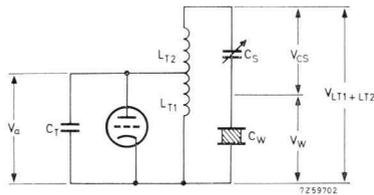
Fig. 6.16. Schematic of auto-transformer circuit that can be used where  $V_{C_S} + V_w$  must be greater than  $V_a$ . The transformer section  $L_{T1} + L_{T2}$  could, for very high frequencies, also take the form of a line.
