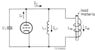
Fig. 6.5. Diagram of parallel connected load coil.  $L_W$  will generally be of a greater inductance than  $L_T$  and may be made interchangeable. The useful load coil current  $I_W = I_C - I_T$  will depend on the ratio of the inductive values of  $L_T$  and  $L_W$ .
