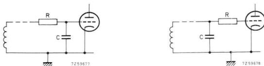
*Fig. 5.42. The diagrams show simple RC suppressors used when fundamental and parasitic frequencies are well separated. The resistive component need often be no more than a nickel alloy strip with a d.c. resistive value of a fraction of an ohm and therefore consume only little fundamental power.*
