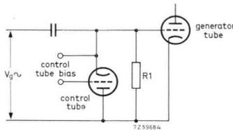
Fig. 5.47. Circuit of tube controlled grid resistor.  $R_1$  is in parallel with the control tube and should have a value several times that required for normal operation. Its purpose is to provide a grid-cathode path for the oscillator tube in case of control circuit failure. The r.f. section of the circuit is not shown.
