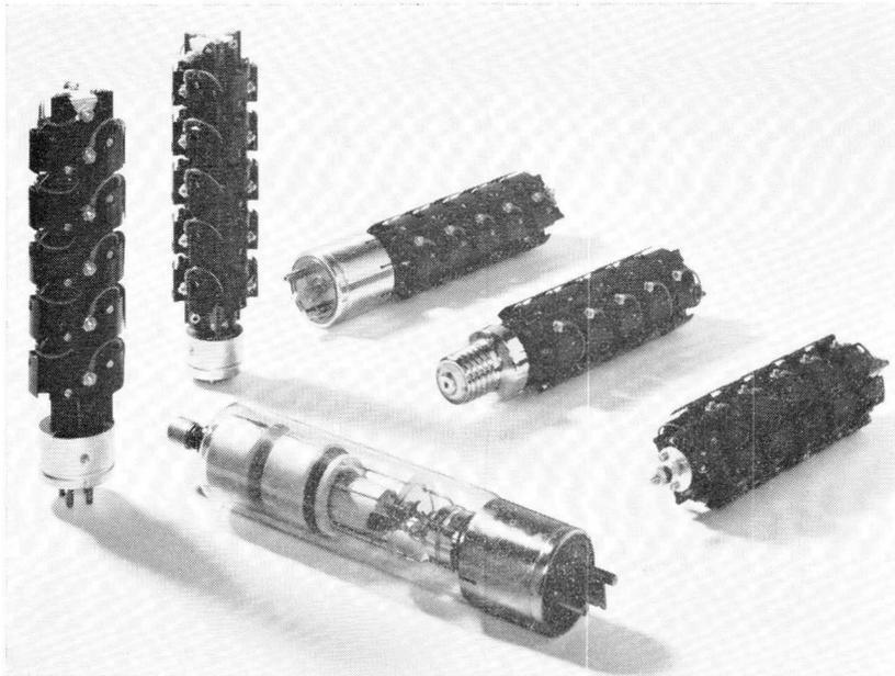
*Fig. 2.1. Solid-state high-voltage rectifier stacks, compared with a gas-filled rectifier diode. Two basic stack mounting arrangements are available — stud mounting and tube-base mounting (for direct replacement of tubes); there are four types of tube-base mounting in our range, as shown.*
