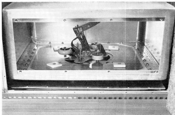
*Fig. 8.11. Tank circuit capacitor box, containing the grid-filament circuit. The large p.t.f.e. sandwich capacitor at the bottom of the box is the grid blocking capacitor. The grid bias lead is connected at the rear left-hand corner and is dressed along the inside of the box for decoupling purposes.*
