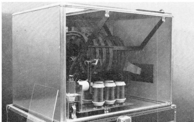
*Fig. 8.2. General view of the equipment. The work coil and load are not visible as they are mounted outside on the right-hand panel.*
