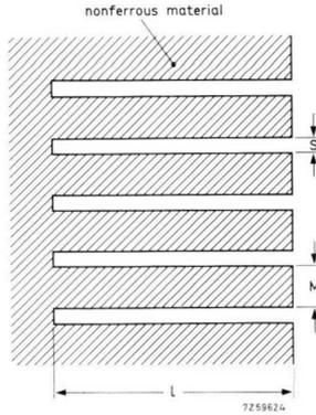
Fig. 4.2. Sketch of Faraday screen. The cross hatched area is the metallic panel out of which the screen has been cut. The mark-space ratio  $M/S$  will determine the degree of higher order harmonic suppression, and the path length along the edges of the whole screen any possible resonant slot properties.  $L$  should be a significant multiple of  $M + S$ .
