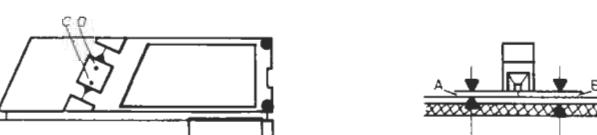
With screws C and D adjust so that distances A and B are identical and the plane portion of the pickup is parallel with the top side of the record.
