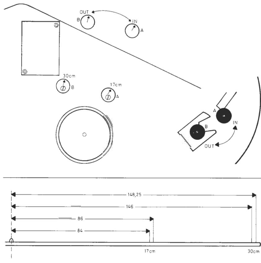
With "45" activated, adjust eccentric A so that the pickup when travelling in automatically will lower into the field marked 17 cm in the sketch above. Eccentric B should be adjusted so that the pickup lowers into the field marked 30 cm with "33" activated.
