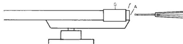
Set the stylus-force adjustment slider to the 0 position.
