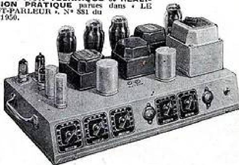
PUISSANCE MODULÉE effective 32 WATTS. Gain 95 db.
