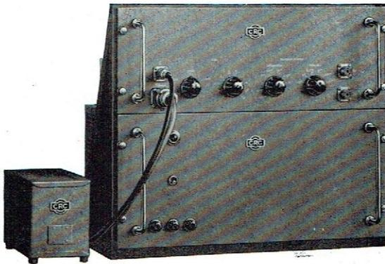
The instrument is designed for linear amplification of negative and positive pulses of small amplitude and consists of three parts : preamplifier - amplifier - power supply unit.
