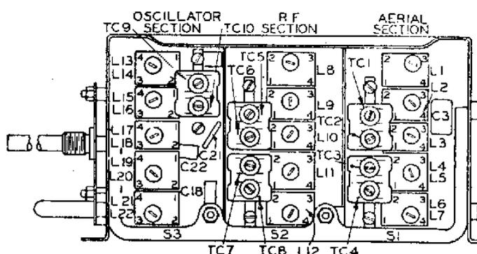
**ABOVE:** Layout of underside of receiver chassis, showing location of major components.
