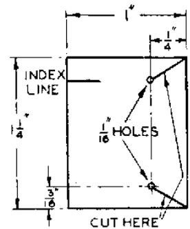
Diagram shows dimensions for auxiliary pointer for use in re-aligning receiver (see Alignment Procedure on Page 4). The pointer can be cut from cardboard, and is used in conjunction with the calibration marks on the chassis pulley support.
