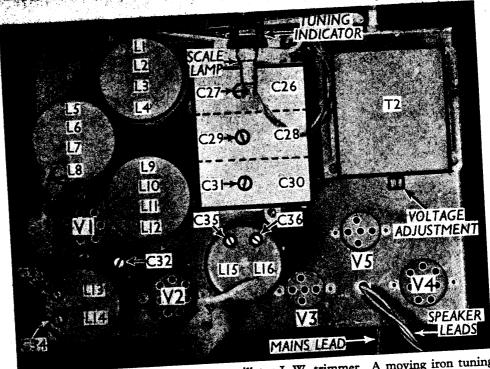
Plan view of the chassis. C32 is the oscillator L.W. trimmer. A moving iron tuning
