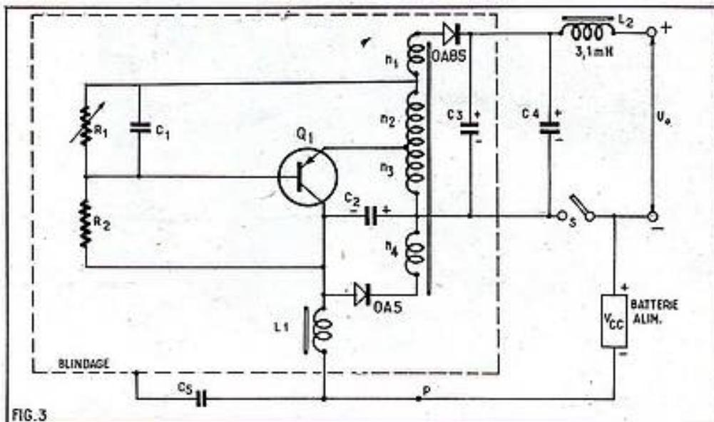
$$V_2 = -n L_2 \frac{di_1}{dt} = -n V_{cc}$$
