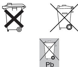
Batteries / accumulators that contain hazardous substances are marked with the symbols on the side. These symbols indicate that it is prohibited to dispose of these batteries in the household waste.
