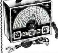
Model 320-K. For service, lab, and school use in FM-AM alignment and to provide TV marker frequencies. Ceramic insulated variable condensers. Highly Stable Hartley oscillator has range of 150 kc to 100 mc with fundamentals to 34 mc. Colpitts audio oscillator supplies pure 400 cycle sine wave voltage for modulation. Large 9" dial. Easy-to-read calibrations. Easily aligned. Complete with tubes. 10" x 8" x 4 3/4". 3-color etched panel. **\$19.95**
