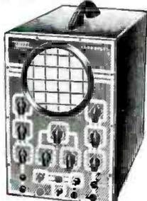
Model 400-K. Laboratory precision scope, for FM, AM & TV servicing. Deflection sensitivity: .65 volts per inch full gain. Horizontal sweep circuit, 15 to 30,000 cycles. Frequency response of horizontal and vertical axis is from 50 to 50,000 cycles. Graticule screen. Operates on 110 to 130 volts AC, 50-60 cycles. 3-color etched, rub-proof panel. Size: 8 1/2" x 17" x 13" high. 3-color etched panel. **\$39.95**
